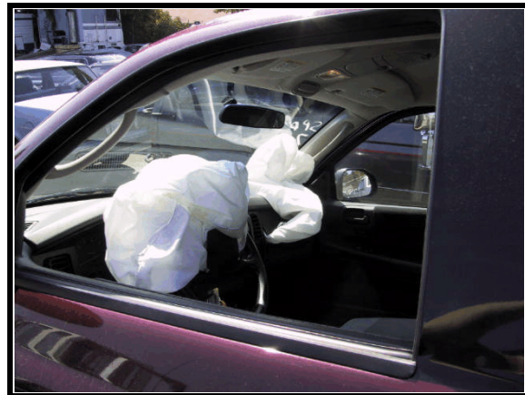
Figure 9. Interior view of Dodge Dakota, showing deployed frontal air bags
