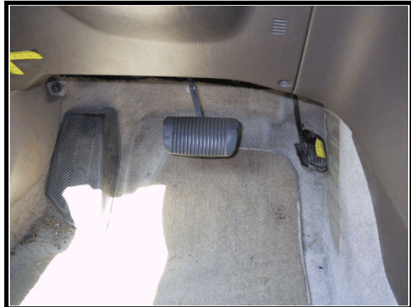
Figure 12. Displaced gas pedal, left knee contact to left instrument panel
