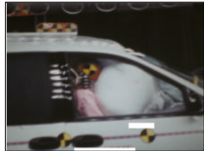
Figure 18. View 21 milliseconds after deployment begins, showing air bag pivoting and engaging the windshield
