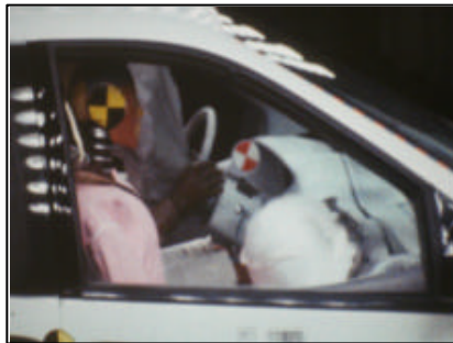
Figure 16. View 4 milliseconds after deployment begins, approximately 20 milliseconds after barrier impact
