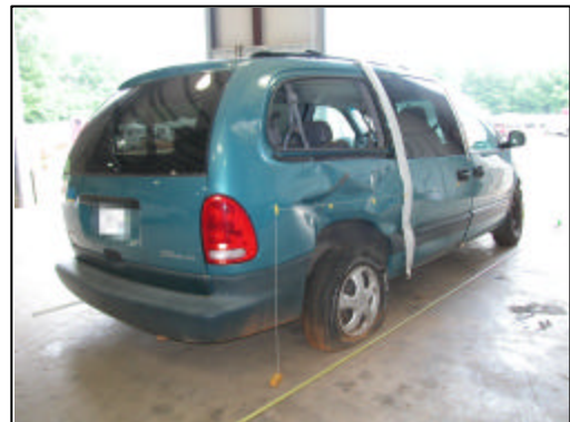
Figure 10. View of right rear side damage from the sideslap
