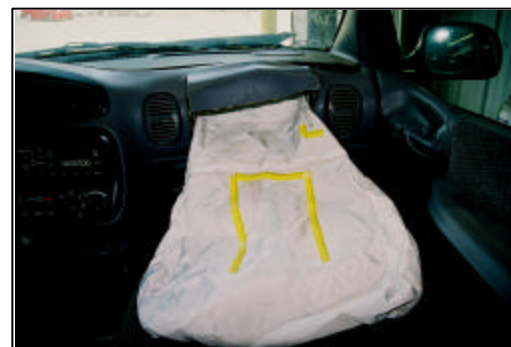
Figure 19. View of top of front right passenger air bag showing area of transfers and membrane tear
