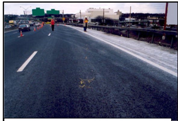
Figure 3: Trajectory of the Jeep evidenced by the RF scratch mark
