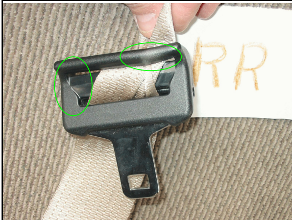
Figure 6: Top of second row right safety belt latch plate; note, guide bar deformed (right) and cinch bar torn and deformed (left) (case photo #44)
