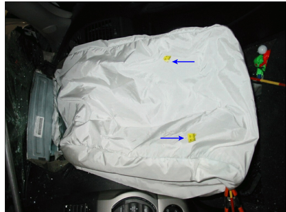
Figure 25: Top surface of case vehicle's deployed front right air bag showing small holes in air bag's fabric, possibly from contact with cracked right windshield's glazing (case photo #51)
