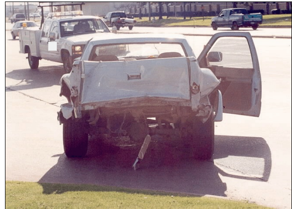
Figure 8: On-scene police photo looking southwest at GMC pickup's back damage from sustained contact impact by Ford SUV; Note: crease line across tailgate of pickup corresponds with Ford's hood deformation (case photo #70)
