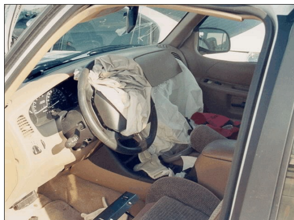
Figure 29: On-scene police photo showing Ford SUV's front seating area and deployed driver and front right passenger air bags (case photo #64)
