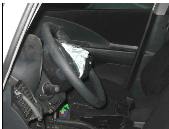
Figure 27: Case vehicle's tilt and telescoping column jammed against instrument panel; Note: no steering wheel rim deformation (case photo #28)
