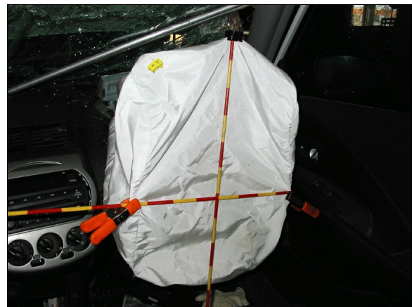
Figure 26: Front surface of case vehicle's deployed front right air bag showing no apparent evidence of occupant contact (case photo #55)
