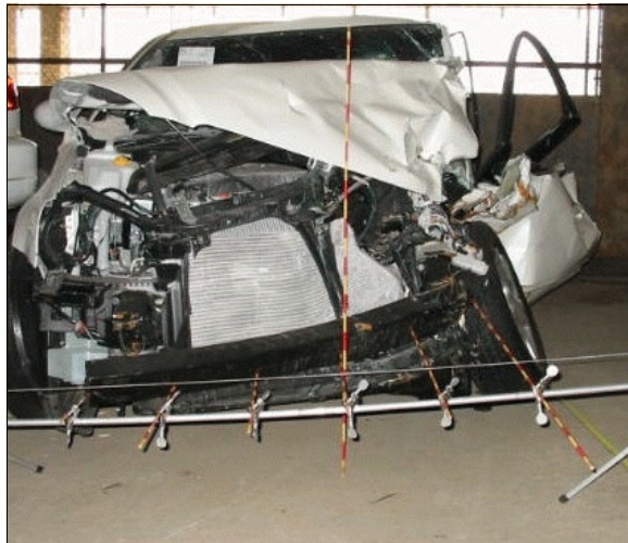
Figure 5: Case vehicle's frontal damage from impacts with GMC pickup and Ford SUV; Note: contour gauge positioned along bumper reinforcement bar (case photo #15)
