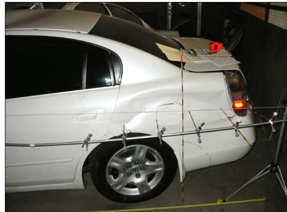
Figure 18: Elevated view of damage to case vehicle's left quarter panel with contour gauge positioned above mid-door level (case photo #22)
