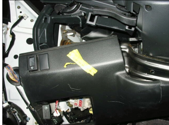
Figure 23: Close-up of occupant contact evidence on left side of case vehicle's driver knee bolster (case photo #34)
