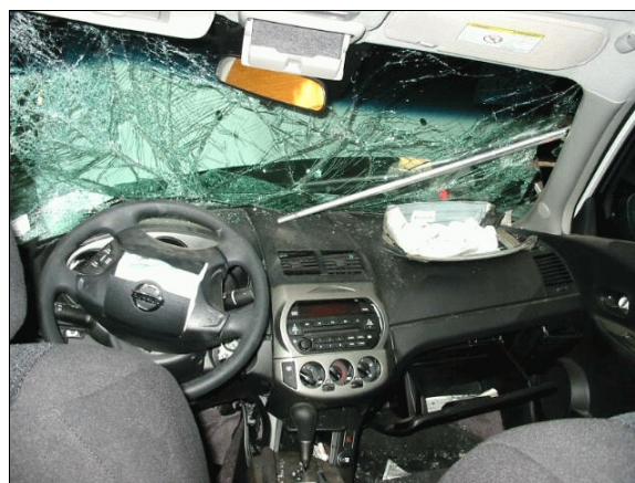
Figure 22: Case vehicle’s front right passenger seating area showing deployed front right air bag, lateral (toward the right) movement of center instrument panel, and no apparent evidence of occupant contact (case photo #37)
