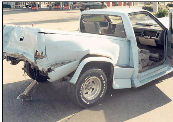
Figure 32: On-scene police photo looking southeast at sustained contact damage to GMC pickup's truck bed from impact by Ford SUV; Note: upward rotation of truck bed was exacerbated during GMC's impact with case vehicle (case photo #71)
