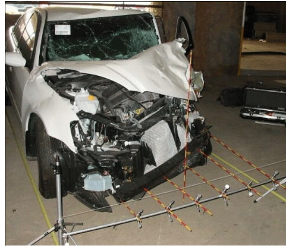
Figure 16: Elevated view of case vehicle's frontal damage viewed from right of front with contour gauge positioned along bumper reinforcement bar (case photo #14)
