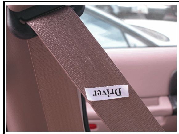
Figure 6. Loading evidence to driver's seat belt
