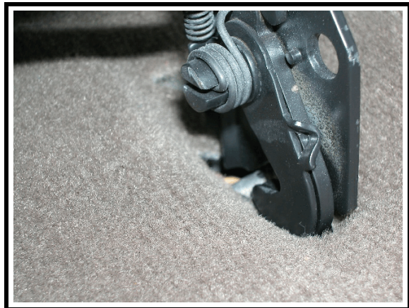
Figure 7. Latch mechanism misalignment
