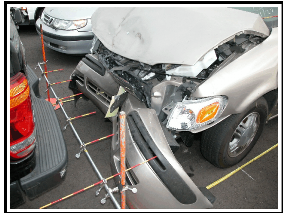
Figure 4. Frontal damage, Chevrolet Venture
