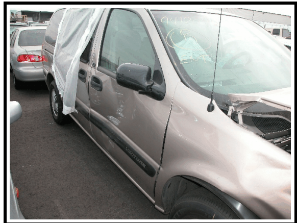
Figure 5. Sideslap damage, Chevrolet Venture
