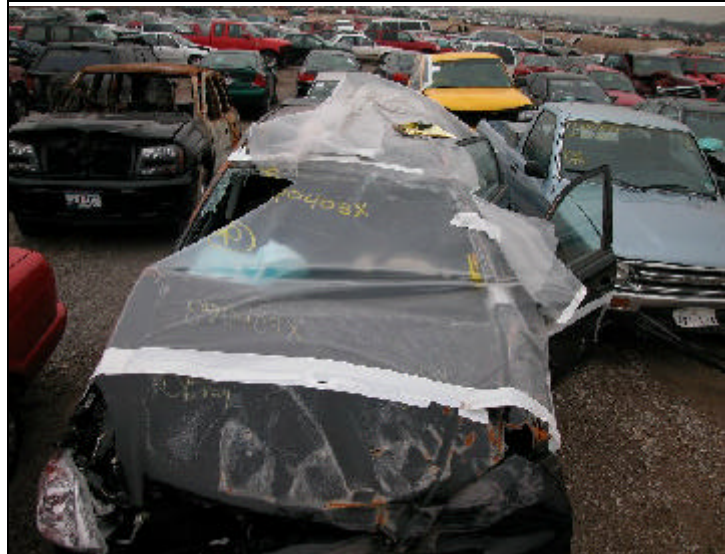
Figure 3. Top of hood, roof, rollover damage
