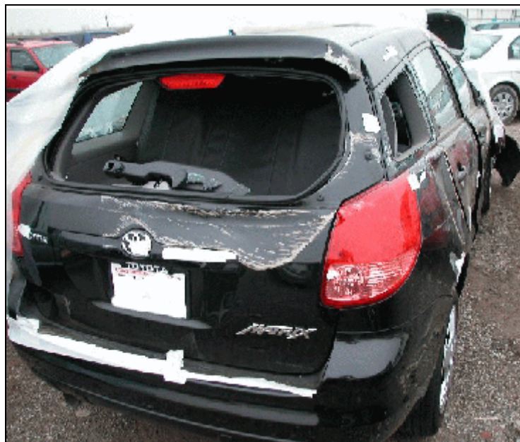
Figure 4. Rear of vehicle—impact with wall
