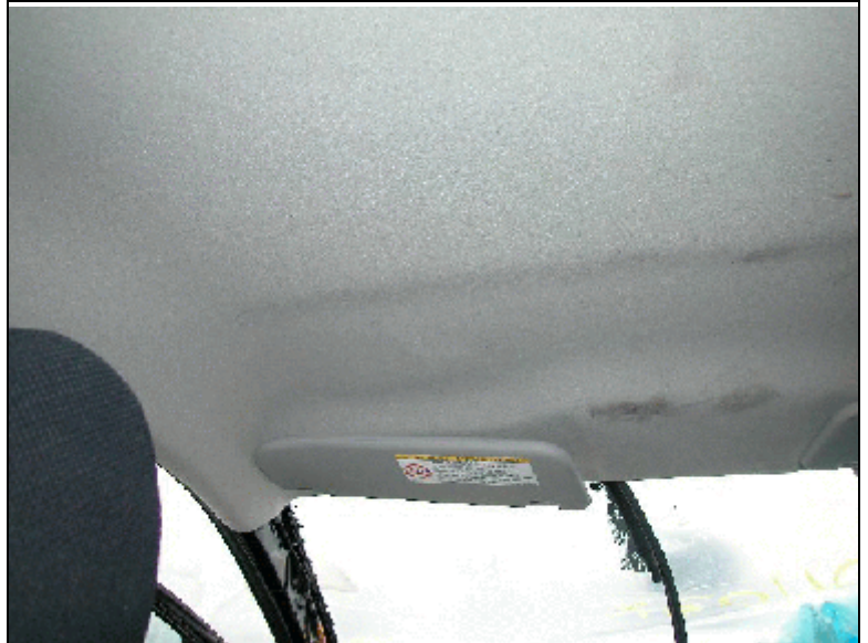
Figure 10. Roof/windshield header (scuffs)
