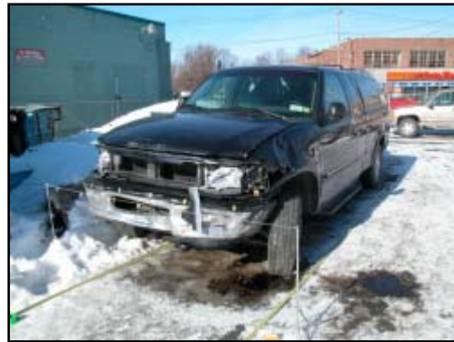
Figure 18. View of front and left side damage on the Ford F-150
