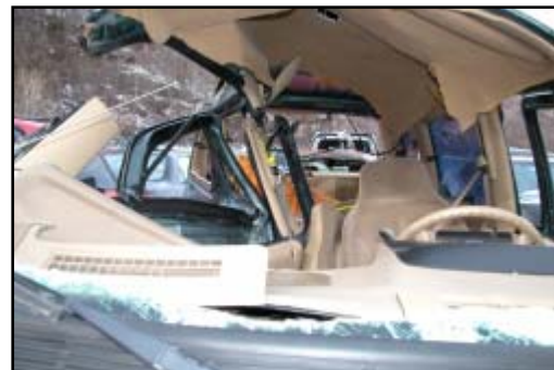
Figure 7. View of interior damage and lateral intrusion
