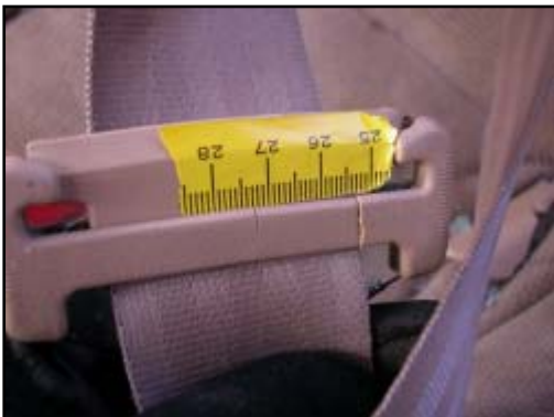
Figure 11. View of fractured rear left latch plate
