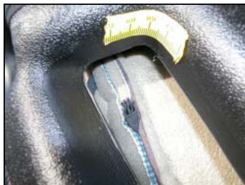
Figure 24. Close-up of abraded left side belt path corner
