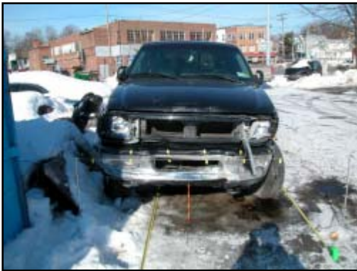
Figure 17. View of frontal damage to the Ford F-150
