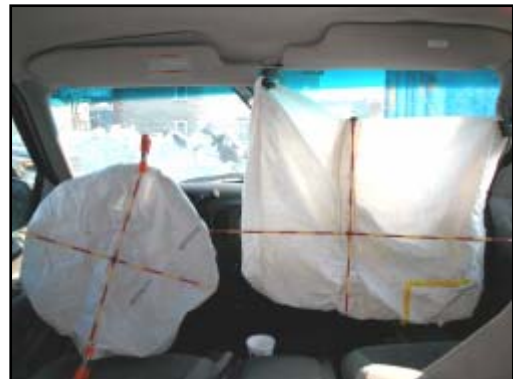
Figure 26. Deployed frontal air bags in the Ford F-150
