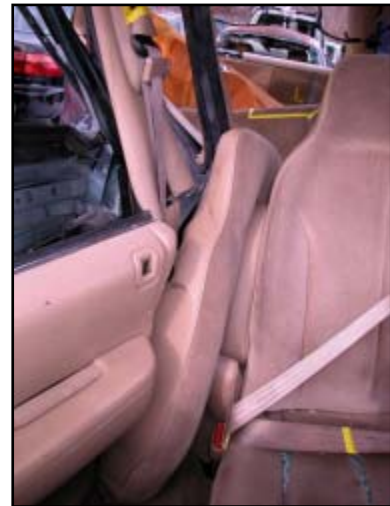
Figure 8. View of deformed front right seat back and intrusion of right front door and right B-pillar
