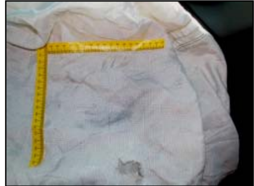
Figure 27. Vinyl transfers and hole on the bottom right aspect of the front right passenger's air bag
