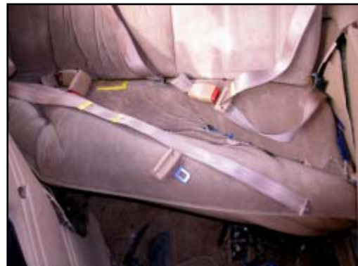
Figure 12. View of rear right safety belt webbing (cut) and latch plate
