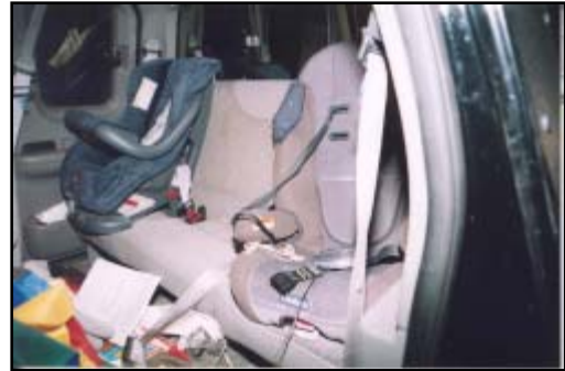
Figure 25. Post-crash photograph showing both CSS in the Ford F-150
