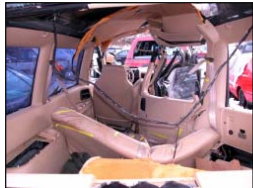
Figure 9. View from the backlight showing intrusion and contacts
