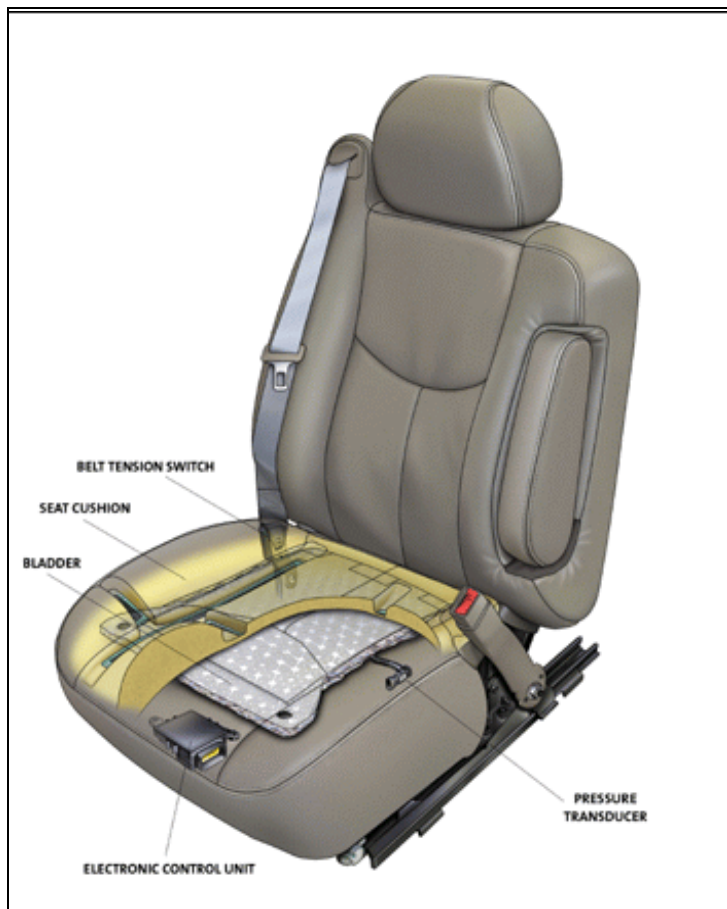
Figure 7. Passenger sensing system (photo from GM web site www.gm.com/company/gmability/safety/images/pss.jpg )
