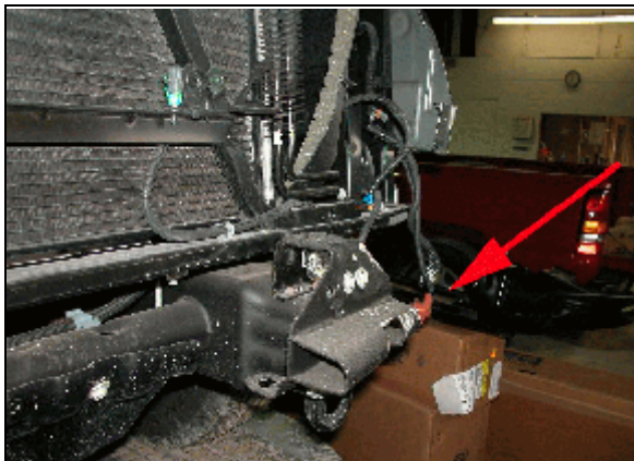
Figure 6. Left bumper mounting bracket—minor scuffing/scratches
