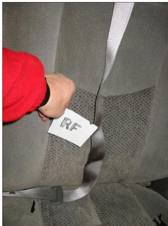
Figure 22: Safety belt webbing for case vehicle's front right passenger showing a wavy pattern indicative of occupant loading (case photo #17)
