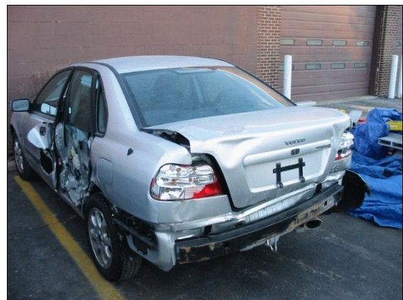
Figure 32: Damage to Volvo's left and back surfaces viewed from left of back; Note: greatest damage to Volvo's back occurred to back right bumper (case photo #64)
