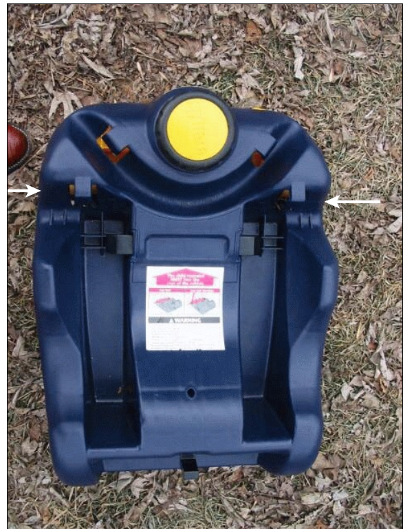
Figure 15: Overhead view of infant child safety seat's detachable base; arrows indicate where case vehicle's safety belts attach through slots in base (case photo #101)
