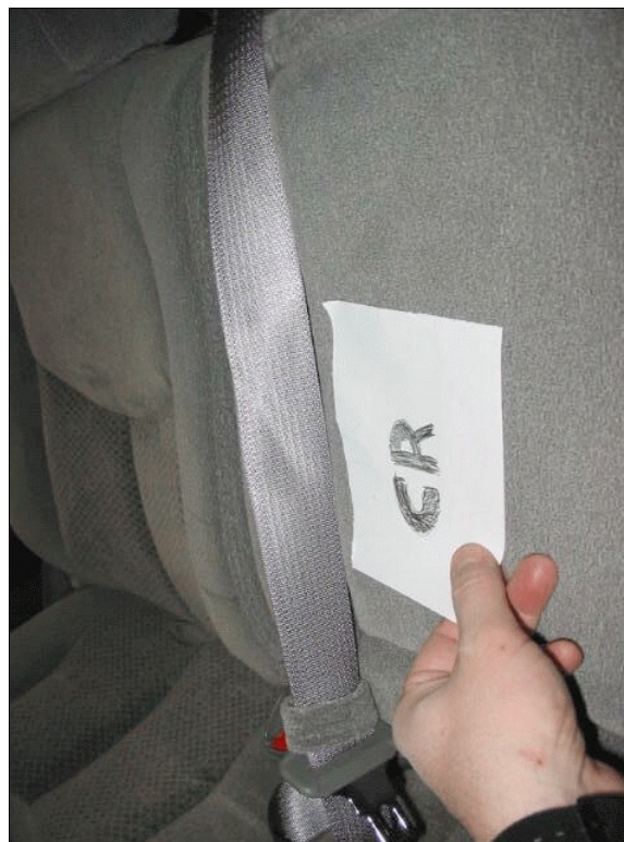
Figure 20: Seat belt webbing for case vehicle's back center passenger showing stress marks indicative of restraint usage (case photo #54)
