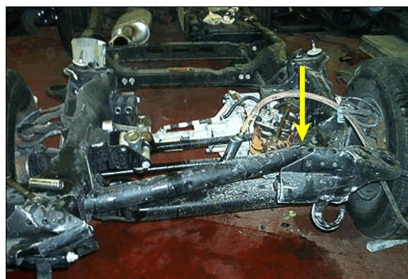
Figure 8: Body shop photo of case vehicle’s frame showing damage to frame’s front cross-member (case photo #113)
