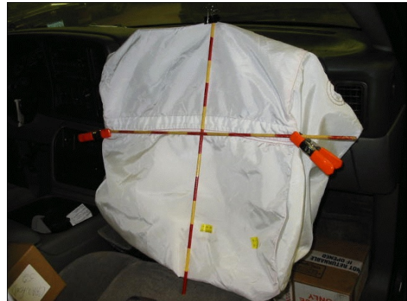
Figure 14: Front surface of case vehicle's deployed front right passenger air bag showing a stain and a scuff in the middle of the lower right quadrant and toward the 6 o'clock position, respectively (case photo #39)
