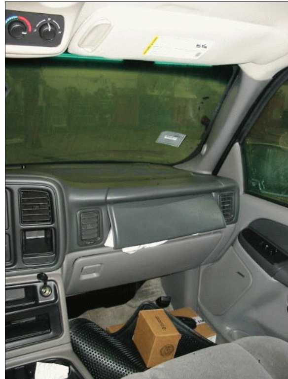
Figure 10: Case vehicle's front right passenger seating area showing no apparent occupant contact evidence to the instrument panel or greenhouse components (case photo #25)
