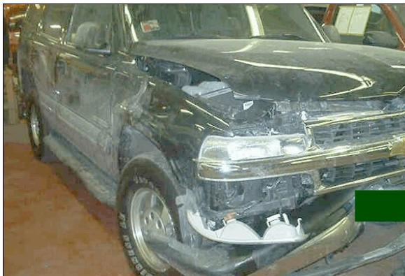
Figure 3: Body shop photo showing case vehicle's front right direct damage and induced damage to right fender and right front door (case photo #109)
