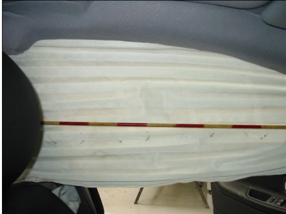
Figure 30: Inboard surface of Volvo's left side inflatable curtain protecting driver's seating area; Note: a hair and a possible lip print were found on the curtain's fabric (case photo #84)
