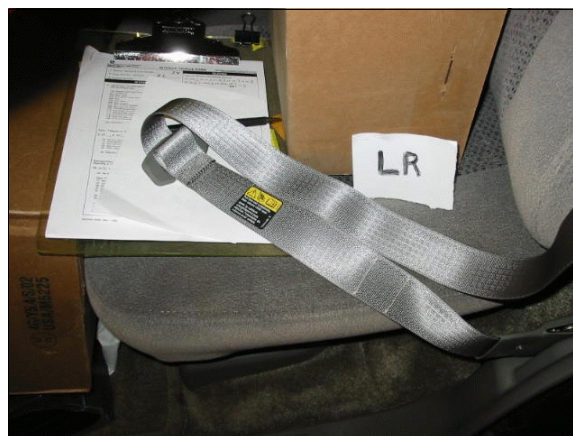
Figure 23: Seat belt webbing for case vehicle's back left passenger showing a wavy pattern indicative of occupant loading (case photo #51)
