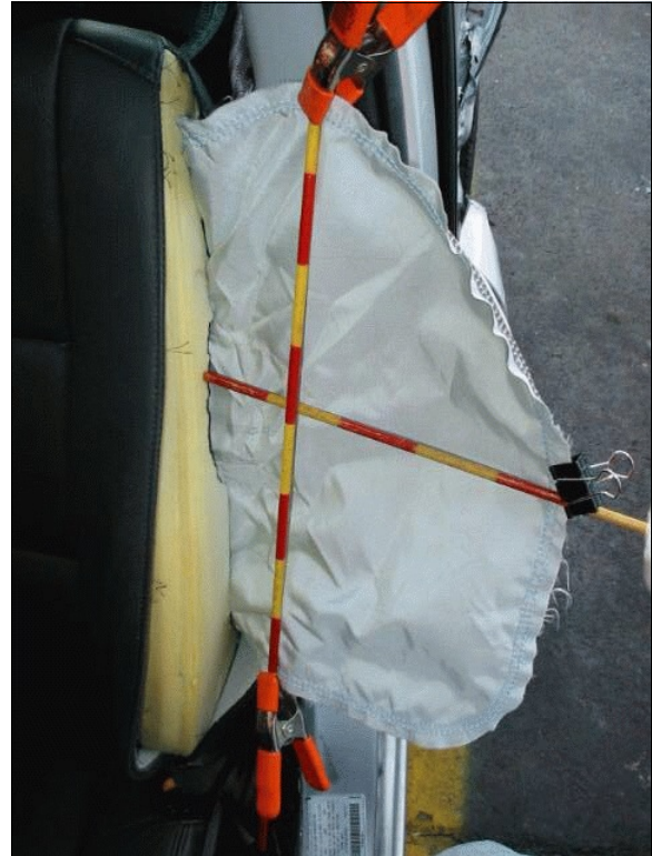
Figure 27: Inboard surface of Volvo's driver seat back-mounted side impact air bag showing no apparent occupant contact evidence (case photo #77)
