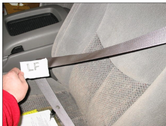
Figure 21: Safety belt webbing for case vehicle's driver showing trace evidence (i.e., slight rippling) of loading (case photo #13)
