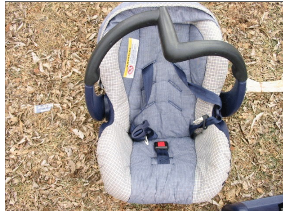
Figure 16: Overhead view of infant child safety seat used by case vehicle’s back center passenger; Note: harness straps positioned through top of three provided slots (case photo #103)
