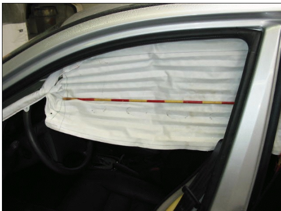
Figure 28: Outboard surface of Volvo's left side inflatable curtain protecting driver's seating area (case photo #78)
