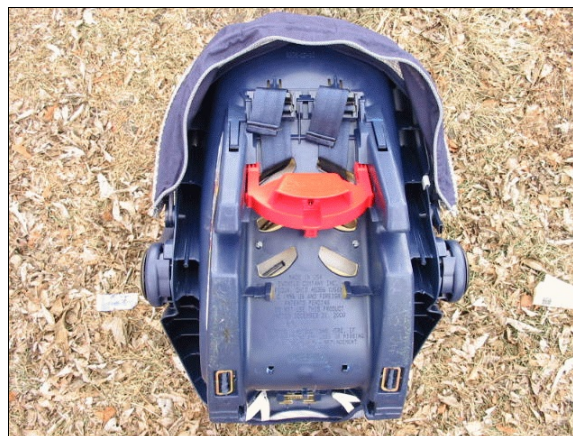
Figure 19: Overhead view of underneath side of shell of infant child safety seat used by case vehicle's back center passenger; Note: no apparent damage (case photo #105)
