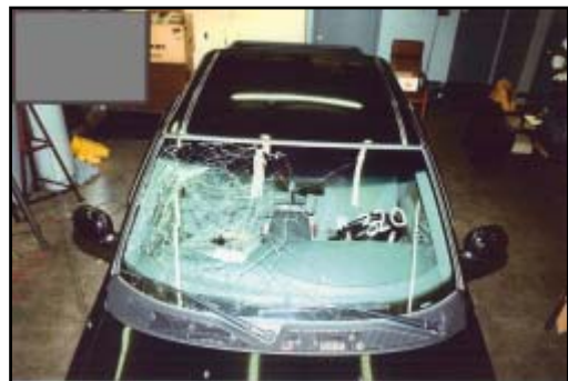
Figure 4. View of fractured windshield
