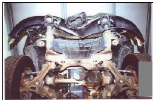
Figure 3. Undercarriage view of damaged Ford F-150
