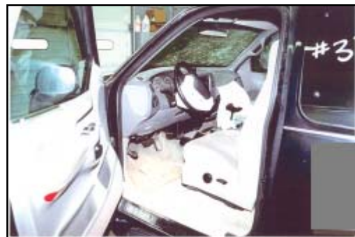
Figure 6. View of frontal air bag system through driver's door
