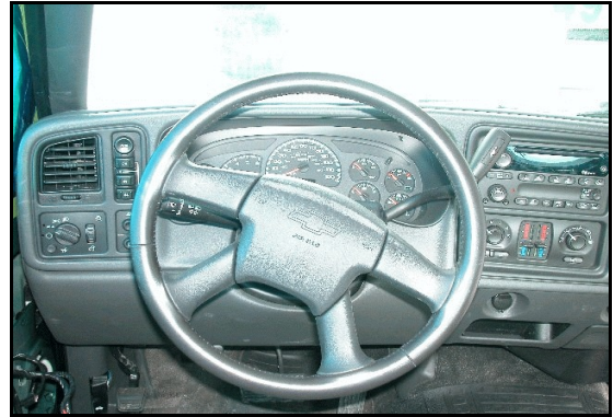
Figure 5. View showing the case vehicle's non-deployed driver's air bag
