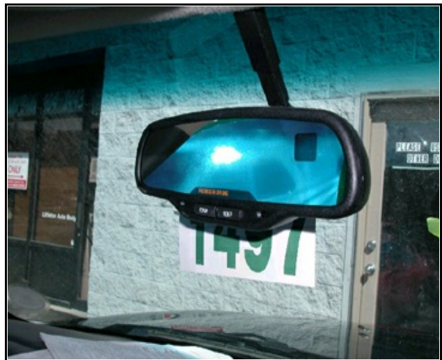
Figure 8. Passenger sensing system indicator
