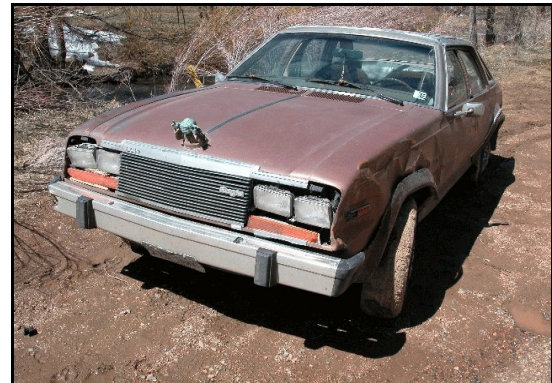
Figure 4. Front left three-quarter view showing left fender damage to other vehicle
