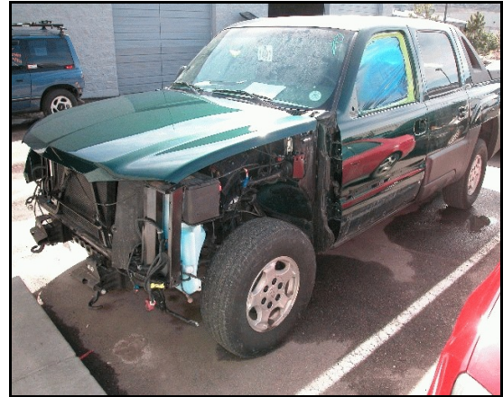
Figure 3. Front left three-quarter view of case vehicle showing vehicle under repair with damaged components removed
