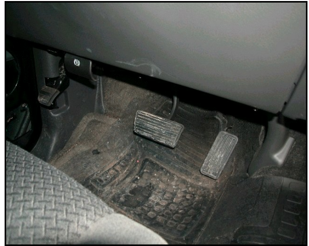
Figure 10. Close-up view showing scuff marks to plastic knee bolster shroud
