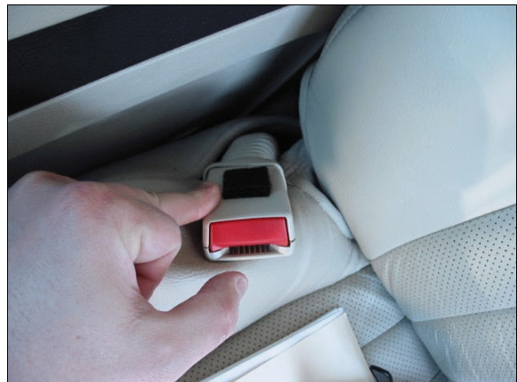
Figure 12: Buckle-mounted pretensioner for case vehicle's driver showing pretensioner actuated (case photo #22)
