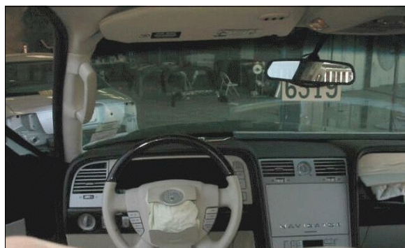
Figure 7: Case vehicle’s driver seating area showing no obvious occupant contact evidence on steering wheel, instrument panel, or greenhouse areas (case photo #20)
