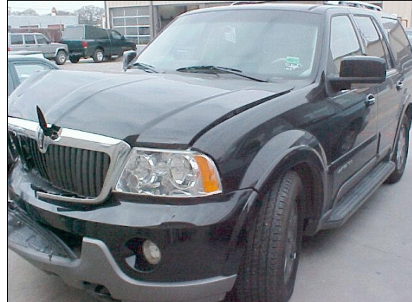
Figure 5: Repair facility photo of case vehicle's frontal damage viewed from left of front, showing that direct damage involved primarily front right half (case photo #10)
