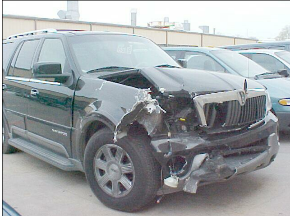
Figure 4: Repair facility photo of case vehicle's frontal damage viewed from right of front, showing damage primarily to front right corner (case photo #16)
