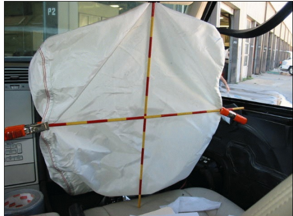
Figure 11: Case vehicle's deployed front right air bag showing no occupant contact evidence (case photo #33)
