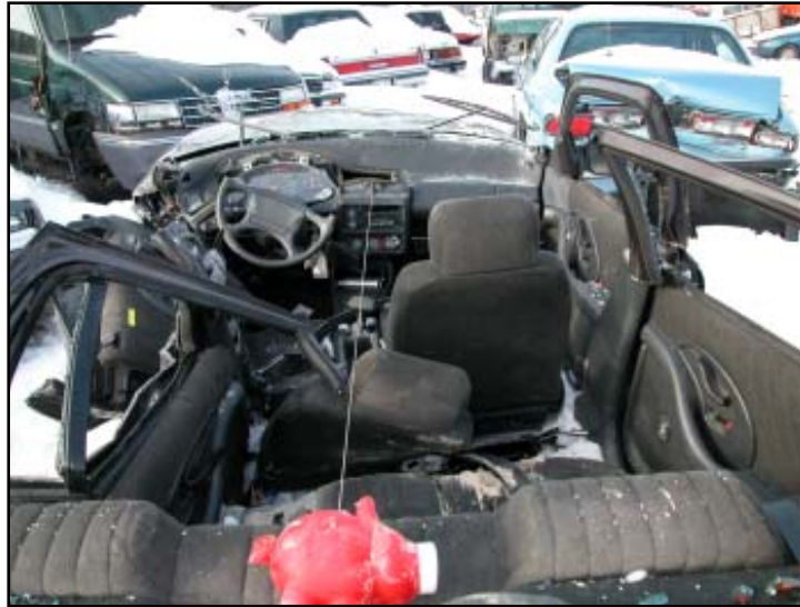
Figure 7. View from rear showing left side intrusions
