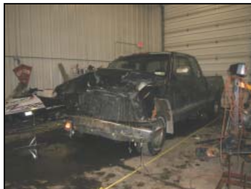
Figure 8. View of frontal damage to the Chevrolet pickup truck
