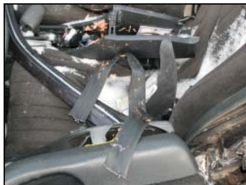
Figure 9. View of cut driver's safety belt
