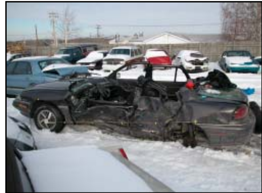
Figure 5. Left side damage to the Grand Am
