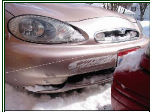
Figure 6. Impact damage to the bumper fascia and air dam.
