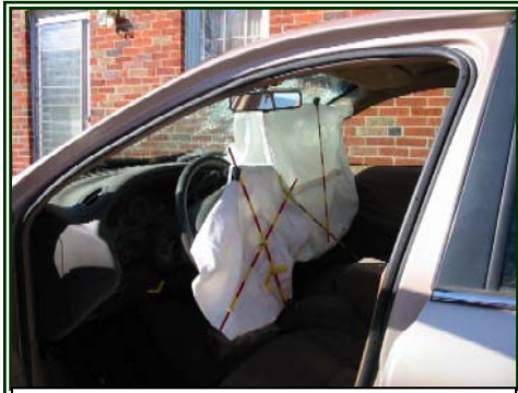
Figure 10. Deployed frontal air bags.
