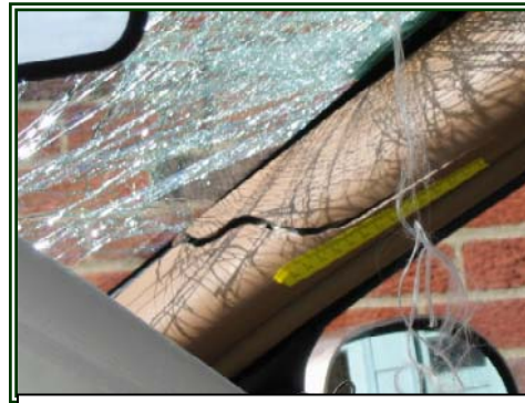
Figure 13. Fractured right A-pillar trim from air bag expansion.
