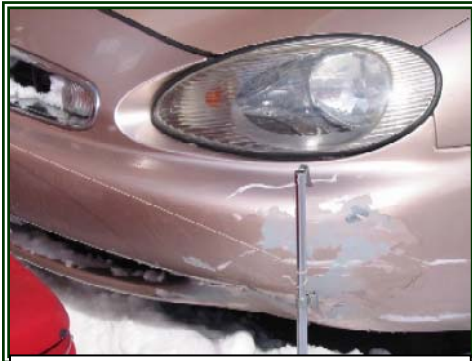
Figure 7. Front left corner damage from porch impact.
