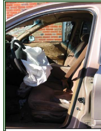
Figure 14. Driver's position and the deployed front left air bag.
