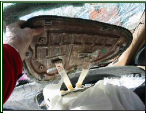
Figure 12. Tethered front right air bag module cover flap.
