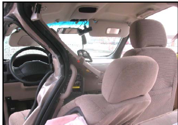
Figure 10: Driver seat deformation and left B-pillar intrusion.
