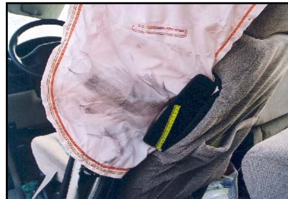
Figure 16: Close-up view of the impeded SAB.
