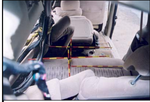
Figure 14: Forward view of the third row intrusion.
