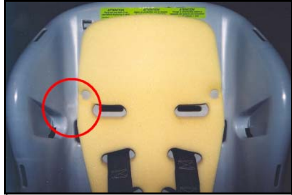
Figure 19: View of plastic stresses to the shell.
