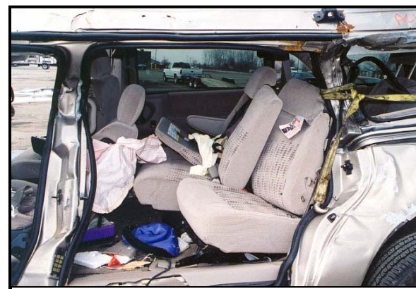
Figure 11 View of the second row seat deformation and intrusion.
