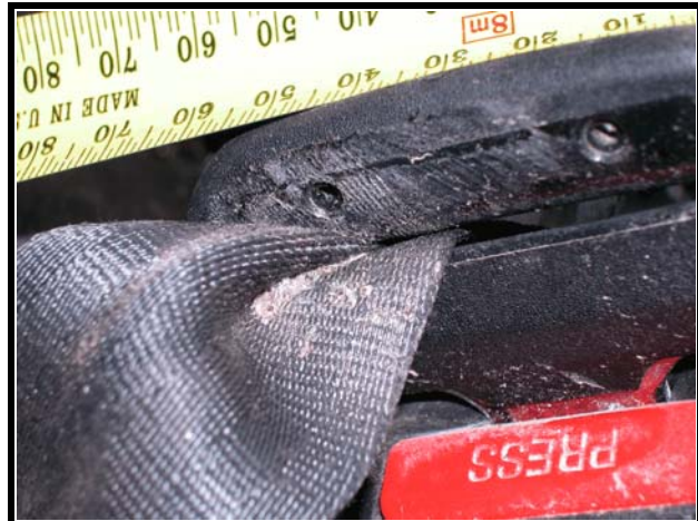
Figure 8. Loading to front right seat belt at latch
