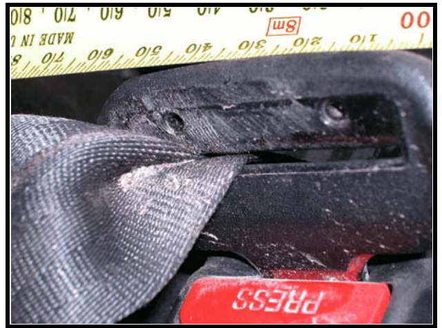
Figure 16. Loading to front right seat belt at latch
