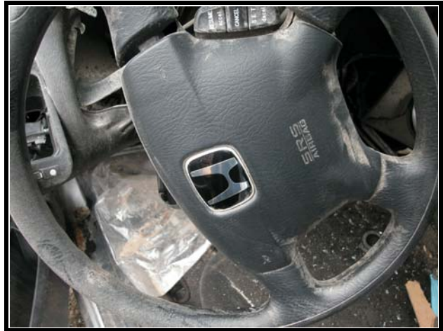
Figure 9. Non-deployment of driver's air bag
