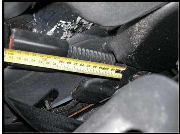
Figure 7. Front right seat belt with no pretensioner compression
