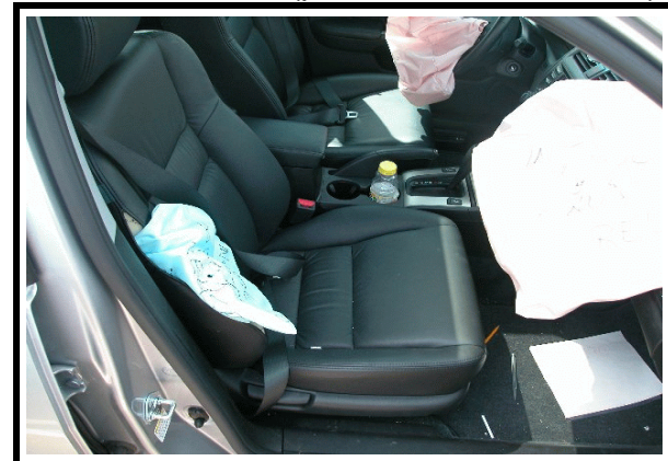
Figure 4. View of front right position showing deployed front and side air bags along with spooled lap and shoulder restraint (pretensioner actuation)
