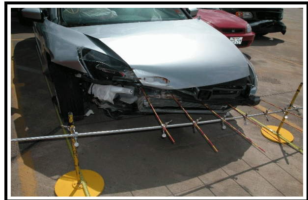
Figure 2. Exterior view showing frontal deformation to case vehicle.
