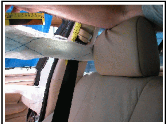
Figure 10. Right ITS (contact evidence to structure and B pillar)
