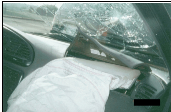
Figure 5: Front right air bag and cover flap, view from right (case photo #10)
