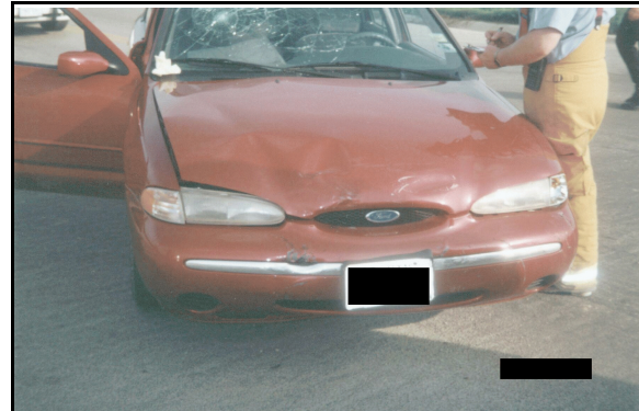
Figure 2: Case vehicle's front at final rest (case photo #04)
