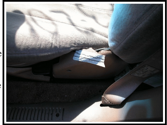
Figure 10. Cracked plastic on driver's seat
