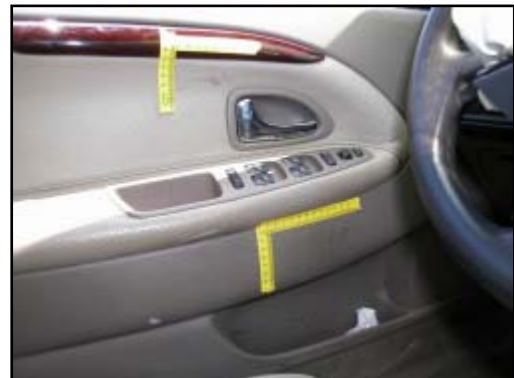
Figure 7. View of scuff marks on driver's door
