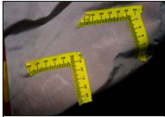
Figure 11. Close-up of white transfers on the front right passenger's air bag
