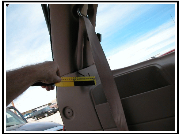
Figure 18. Cracks in D pillar from seat belt loading (third row left)
