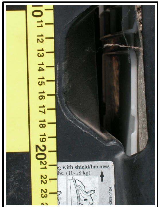
Figure 19. Loading marks to right side of Cosco seat
