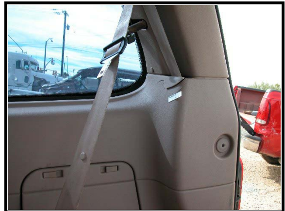
Figure 21. Cracks in D pillar from seat belt loading (third row right)
