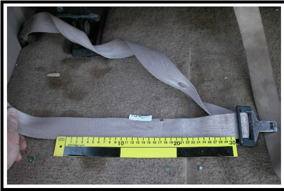
Figure 17. Loading to lap and shoulder belt, left side, third row
