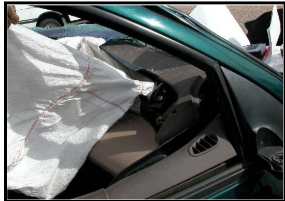
Figure 12. Side view of front right passenger's air bag
