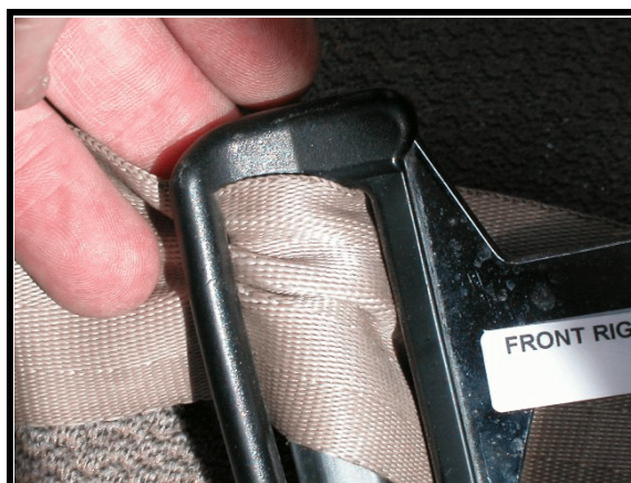
Figure 27. Webbing locked into front right passenger seat belt latch
