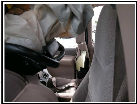
Figure 25. Deformation to bottom of steering wheel rim
