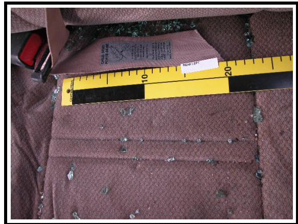
Figure 15. Second row left seat position, shows belt cut by EMS personnel
