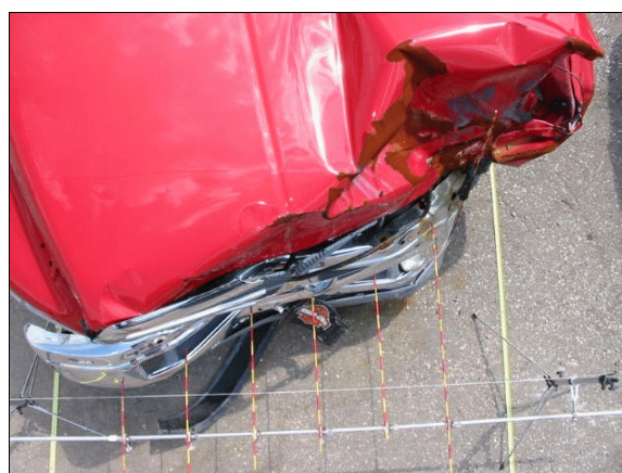
Figure 34: Overhead view of Dodge pickup’s frontal damage with contour gauge set at bumper level (case photo #69)
