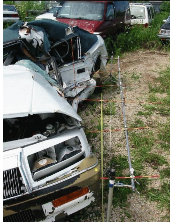
Figure 11: Reference line view from front of case vehicle's left side damage with contour gauge set above sill level (case photo #10)
