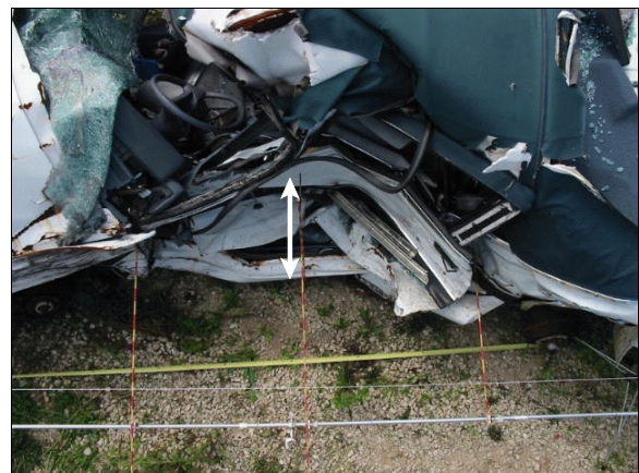
Figure 12: Overhead view of case vehicle's left side damage and crush pocket on driver's door; Note: arrows indicate difference between crush at sill and crush above sill level (case photo #22)
