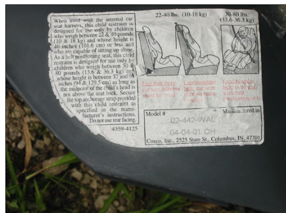
Figure 26: Instructions on Cosco child safety seat providing information pertaining to make/model, height/weight restrictions, and integration of vehicle's safety belts with child seat (case photo #58)
