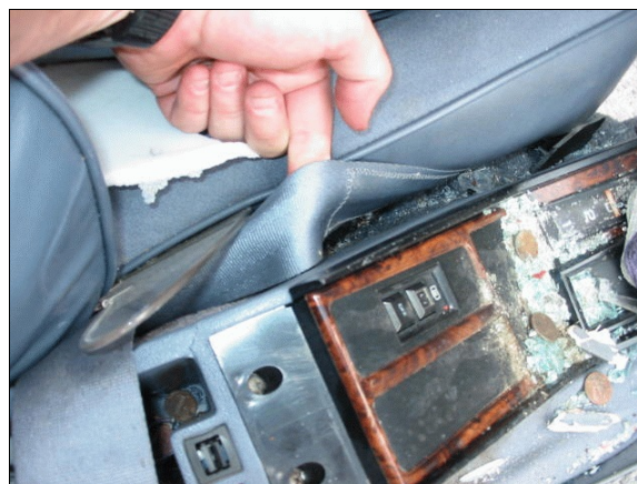
Figure 30: Webbing from case vehicle driver's automatic, shoulder belt showing webbing lodged between intruded driver seat and center console, indicating webbing not in use at time of crash (case photo #44)
