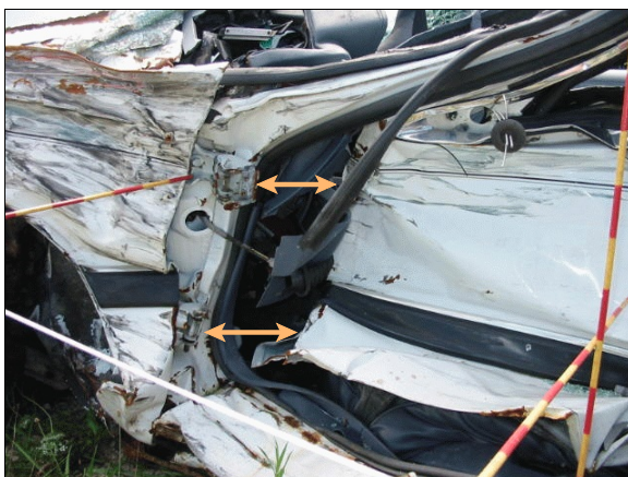
Figure 15: Close-up of door hinge failure (arrows) on case vehicle’s driver door (case photo #25)
