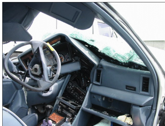
Figure 29: Case vehicle's front right passenger seating area showing extensive intrusion to instrument panel and contact to steering wheel rim; Note: no apparent evidence of occupant contact to either center or right instrument panels (case photo #33)
