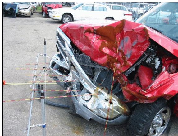
Figure 33: Reference line view from left with contour gauge at bumper level showing Dodge’s oblique crush profile and damaged and restricted left front tire (case photo #62)
