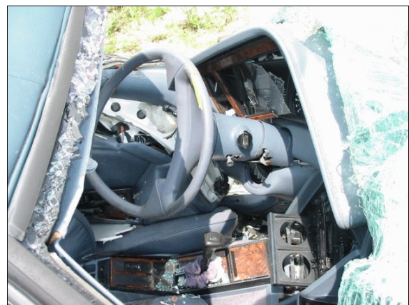
Figure 21: Overhead view of case vehicle's steering column and center console; Note: damage to steering column, steering wheel rim and hub, holed windshield's glazing, and intrusion of driver's seat onto center console (case photo #36)
