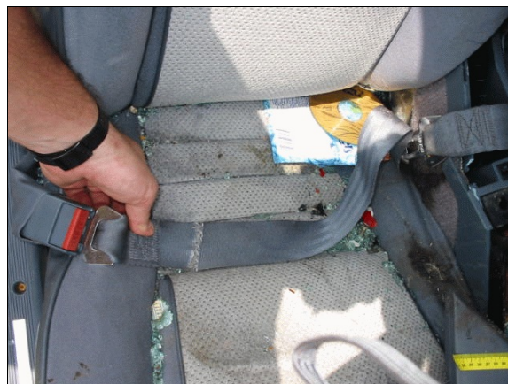
Figure 27: Overhead view of case vehicle's manual, front right lap belt which was used to secure Cosco child safety seat used by front right passenger (case photo #46)
