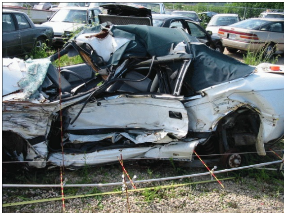
Figure 10: Case vehicle's left side damage from left "A"-pillar rearward with contour gauge set at sill level (case photo #13)
