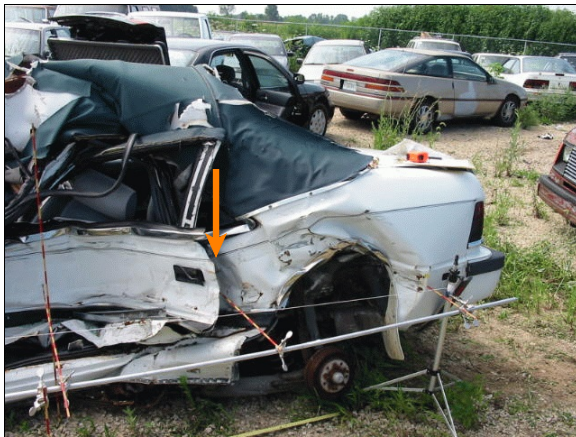
Figure 13: Case vehicle’s left side damage from left “A”-pillar rearward with contour gauge set above sill level; Note: arrow indicates door latch failure (case photo #16)
