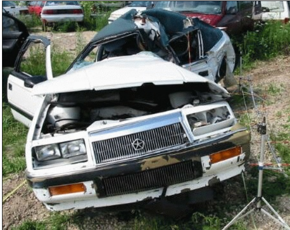
Figure 6: Case vehicle's left side impact viewed from front showing leftward shift (case photo #08a)
