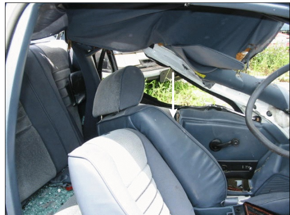
Figure 20: Case vehicle's front seating area viewed from right showing twisted driver's seat, distorted steering wheel rim, contact to left "A"-pillar, and hidden (arrow) contact to side door panel; Note: front right head restraint missing (case photo #45)
