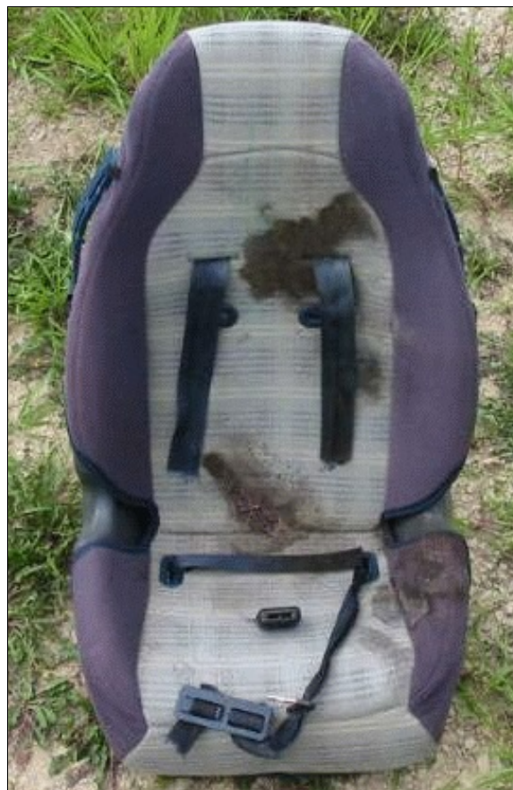
Figure 22: Frontal view of Cosco forward-facing, high-back, combination child seat-configured with five-point harness, used by case vehicle's front right passenger showing harness straps cut by rescue personnel (case photo #47)
