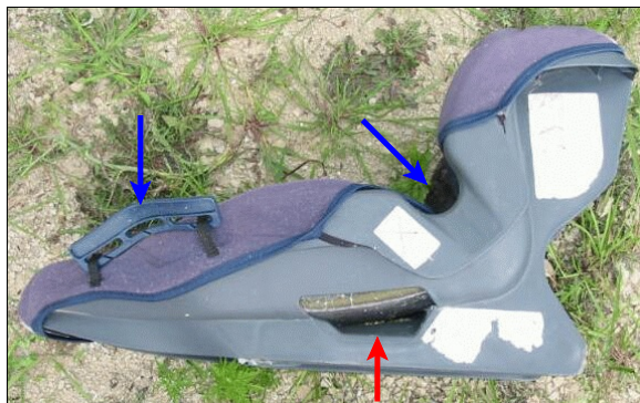
Figure 25: Overhead view of Cosco child safety seat's right side showing locations for securing vehicle's safety belts when seat used as forward-facing seat (red arrow) with harness straps or as belt-positioning booster seat (blue arrows) without harness straps (case photo #50)
