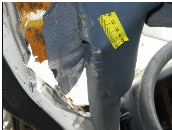
Figure 32: Close-up of contact evidence on case vehicle's left "A"-pillar deposited by case vehicle's driver; Note: hair on "A"-pillar (case photo #39)
