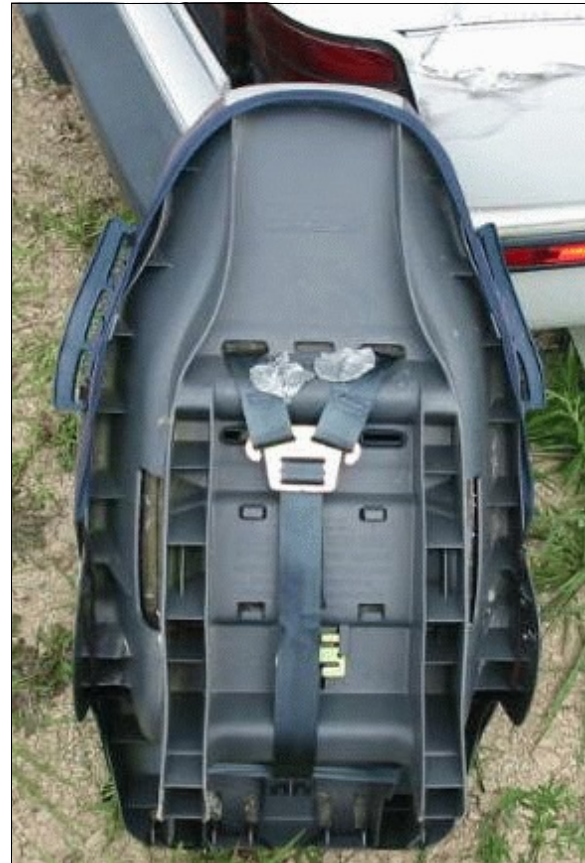
Figure 24: Back surface of Cosco child safety seat showing harness straps positioned through upper slots and no apparent damage to child seat; Note: locking clip secured on seat back (case photo #55)
