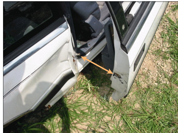
Figure 16: Overhead view of case vehicle’s right front door which was pried open (arrows) by rescue personnel (case photo #29)
