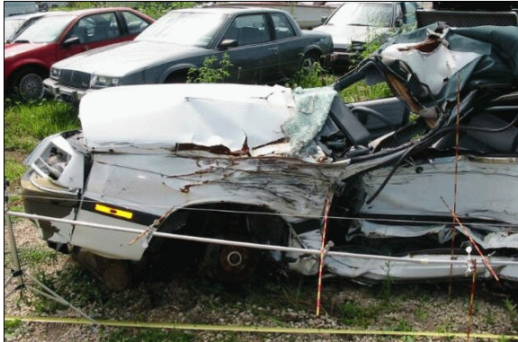
Figure 9: Case vehicle's left side damage forward of left "B"-pillar with contour gauge set above sill level; Note: initial contact with Dodge began forward of front axle (case photo #12)
