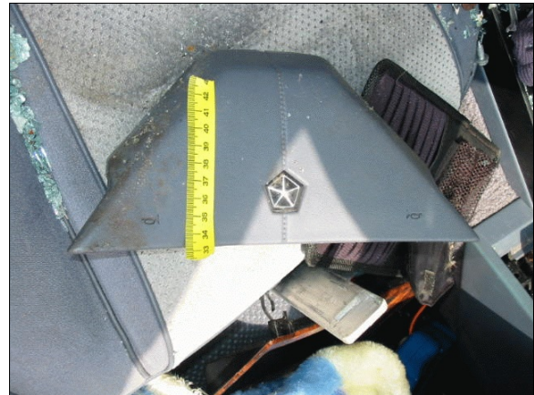
Figure 19: Overhead view of plastic piece that covered case vehicle's steering wheel hub showing evidence of occupant contact (case photo #42)
