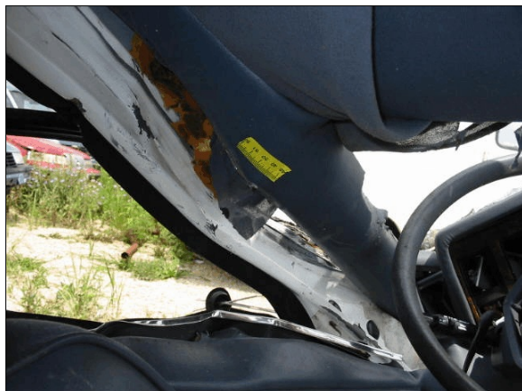
Figure 31: Contact evidence along case vehicle's left "A"-pillar deposited by case vehicle's driver (case photo #38)
