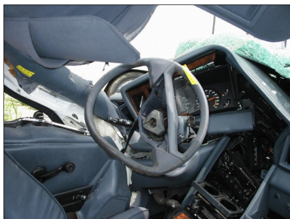
Figure 17: Case vehicle’s driver seating area showing extensive intrusion and contact evidence on steering wheel rim and left “A”-pillar; Note: top of rim is toward 9 o’clock position and plastic cover for wheel hub is absent (case photo #32)
