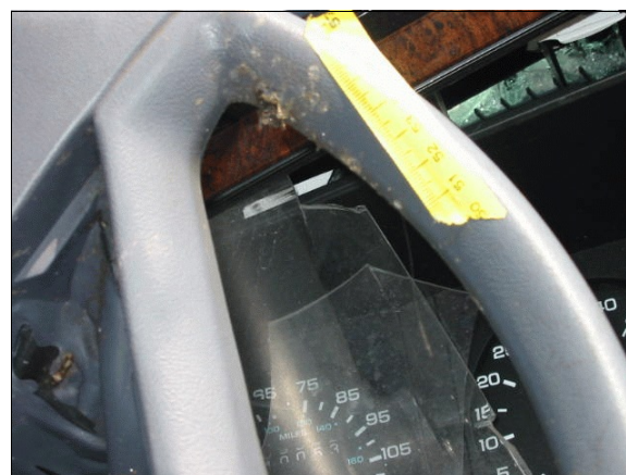
Figure 18: Close-up of contact evidence on case vehicle’s deformed steering wheel rim (case photo #37)
