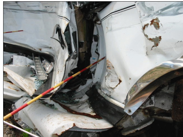
Figure 14: Close-up of door latch failure on case vehicle’s driver door (case photo #24)
