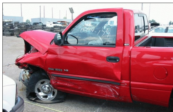
Figure 35: Dodge pickup’s side slap damage from left front of case vehicle; Note: damaged, deflated left front tire and induced damage (rearward movement) to driver’s door from frontal impact (case photo #63)
