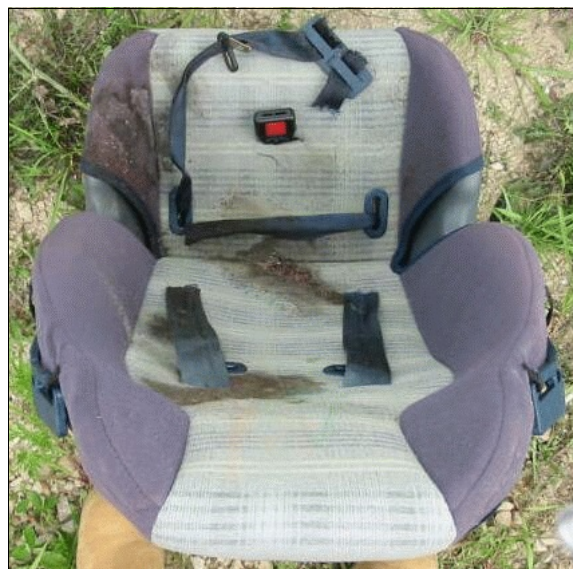
Figure 23: Overhead view from back of Cosco child safety seat used by case vehicle's front right passenger; Note: harness straps cut by rescue personnel (case photo #48)
