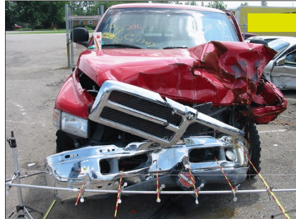
Figure 7: Dodge pickup's frontal damage from impact with case vehicle left side; Note: greatest crush occurred at front left corner (case photo #59)
