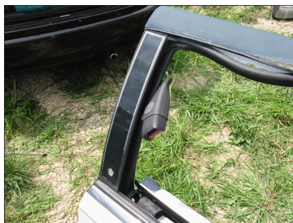
Figure 28: Case vehicle's right front door showing door-mounted buckle for non-motorized front right shoulder belt (case photo #46a)
