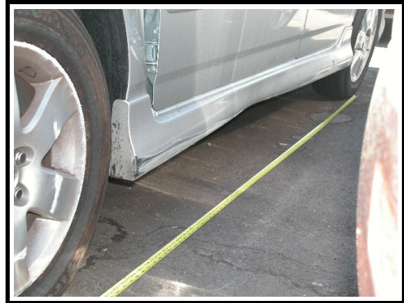
Figure 5. Left side sideswipe damage to left front rim and sill
