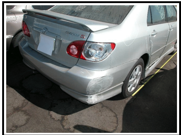
Figure 4. View showing wall contact damage to the right rear bumper fascia
