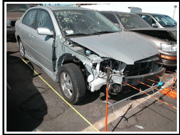
Figure 1. Front right, three-quarter view showing corner impact with continuous right plane sideswipe
