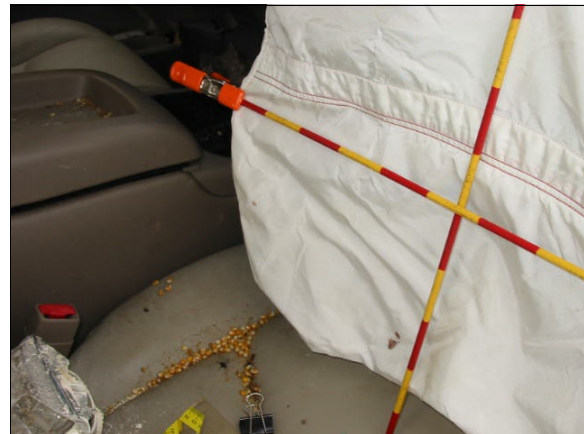
Figure 23: Close-up of blood spot at 6 o'clock position on front surface of case vehicle's deployed front right passenger bag (case photo #51)
