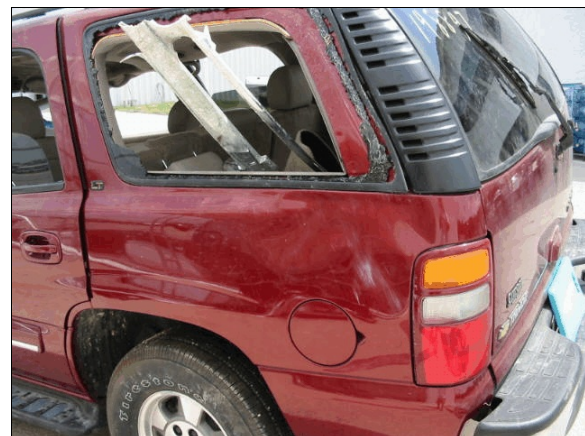
Figure 7: Close-up of case vehicle's left quarter panel showing side slap damage approximately between gas tank filler cap and window sill; Note: disintegrated glazing (case photo #16)
