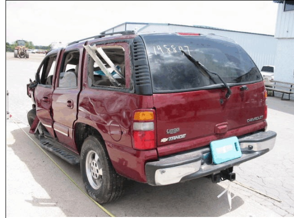
Figure 6: Side slap damage to case vehicle's left quarter panel viewed from left of back; Note: disintegrated glazing (case photo #17)
