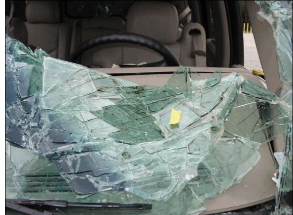
Figure 19: Case vehicle's collapsed windshield glazing showing (yellow tape) blood stains on glazing (case photo #49)
