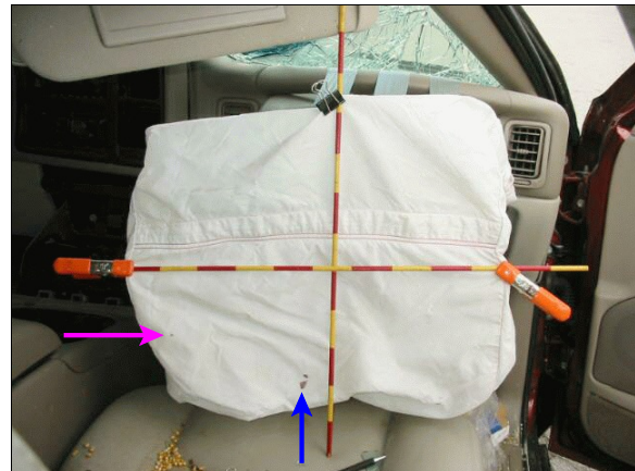
Figure 22: Case vehicle's deployed front right passenger air bag showing two blood spots (arrows) on left lower quadrant of bag's front surface (case photo #50)
