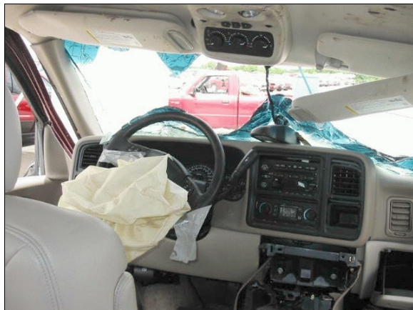
Figure 14: Case vehicle's driver seating area showing deployed driver air bag, collapsed windshield's glazing, and blood splatter on driver's sun visor and across roof (case photo #31)
