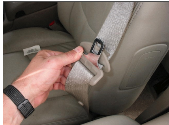
Figure 20: Latch plate for case vehicle's driver safety belt and location of driver's non-deployed seat back-mounted side impact air bag (case photo #45)
