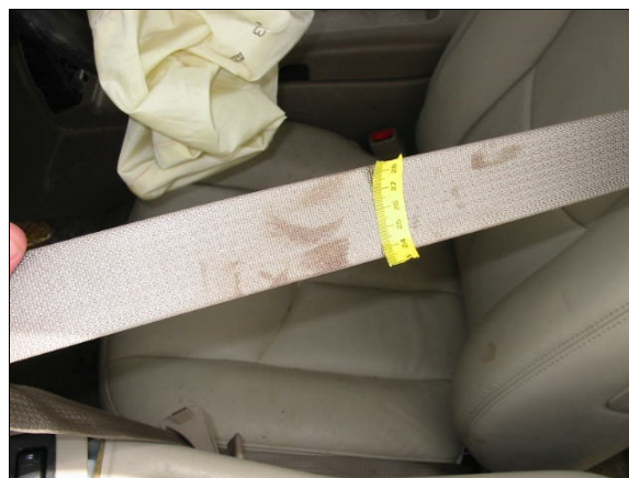
Figure 24: Blood stains on shoulder portion of case vehicle's driver safety belt (case photo #43)
