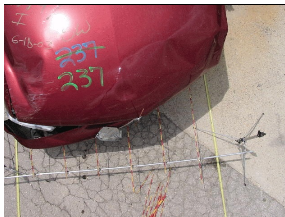
Figure 11: Overhead view of case vehicle’s frontal damage with contour gauge set at bumper level (case photo #27)
