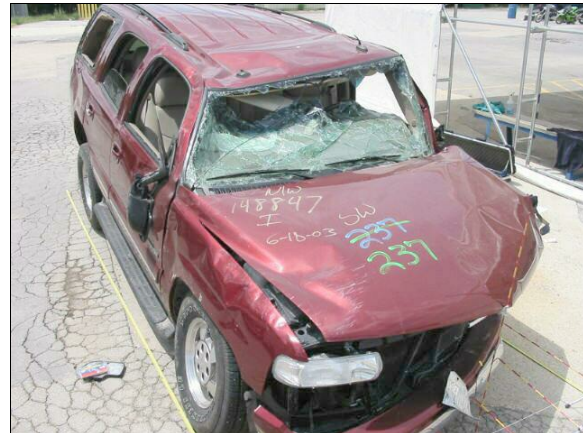
Figure 13: Elevated view from right of front showing case vehicle’s right side and top rollover damage (case photo #25)
