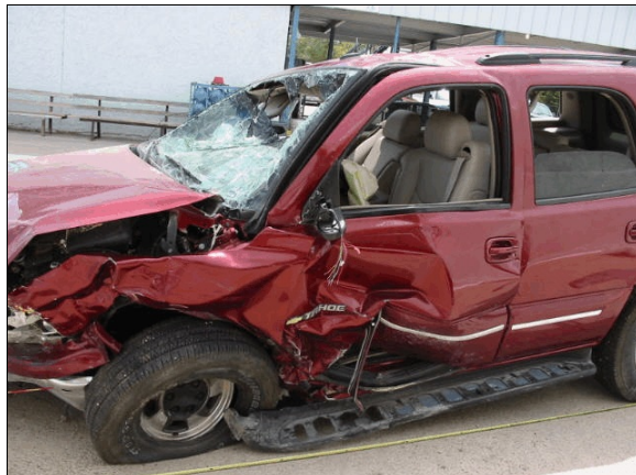
Figure 12: Inward crush to case vehicle’s left fender and left front door which occurred when Hyundai wrapped around during initial impact; Note: driver’s integrated, lap-and-shoulder safety belt system (case photo #15)
