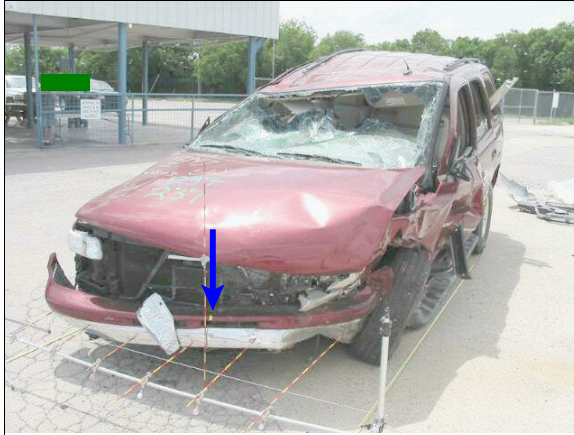
Figure 5: Case vehicle's front and rollover damage viewed from left of front; Note: contour gauge present at bumper level and yellow tape (arrow) indicates end of direct damage area along bumper from impact with Hyundai (case photo #11)
