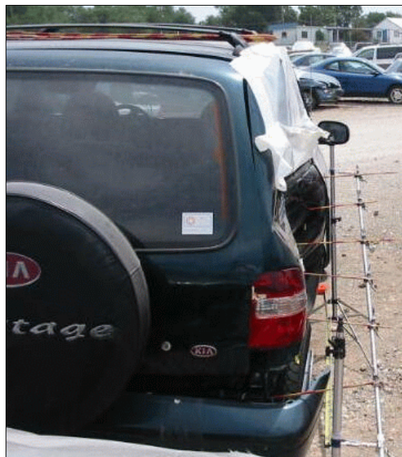
Figure 17: Reference line view from back showing Kia’s right side damage with contour gauge positioned above sill level (case photo #40)
