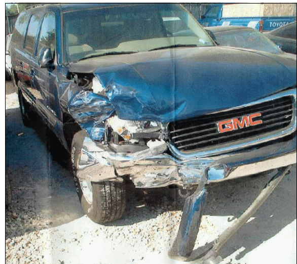
Figure 5: Insurance company photo of case vehicle's front right and corner damage (case photo #14)
