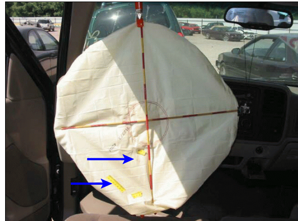
Figure 14: Case vehicle's deployed driver air bag showing occupant contact evidence (i.e., arrows) on air bag's front surface in lower left quadrant near 7 o'clock position (case photo #25)
