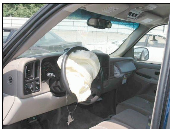
Figure 9: Case vehicle’s front seating area viewed from outside driver’s door showing deployed front air bags and no contact evidence on driver’s knee bolster or instrumental panel or left “A”-pillar (case photo #16)
