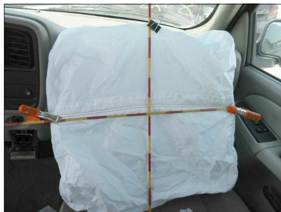
Figure 16: Case vehicle's deployed front right passenger bag showing no apparent contact evidence on air bag's front surface (case photo #30)
