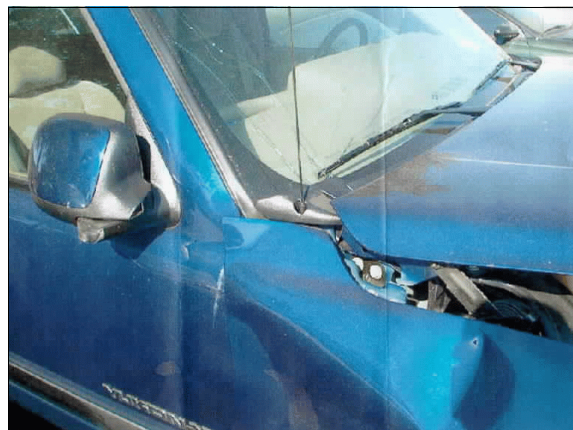
Figure 8: Close-up of induced damage to case vehicle’s right fender, right outside rearview mirror, right “A”-pillar, and the right side of the windshield’s glazing (case photo #08)
