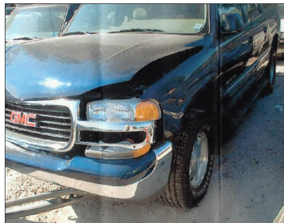
Figure 7: Insurance company photo of induced damage to case vehicle's left front corner (case photo #13)
