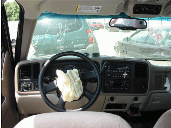
Figure 10: Case vehicle's driver seating area showing deployed driver air bag and no apparent evidence of occupant contact to left or center instrument panels or greenhouse area (case photo #19)
