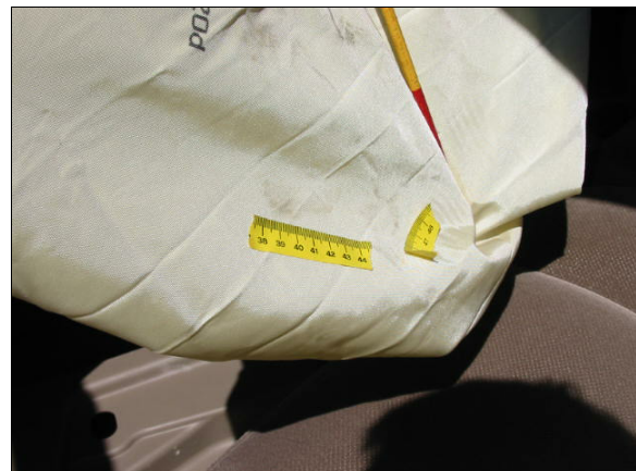
Figure 15: Close-up of contact evidence (i.e., smudges) near 7 o'clock position of case vehicle's deployed driver air bag (case photo #26)
