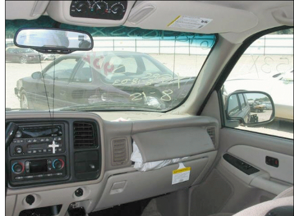
Figure 11: Case vehicle's front right passenger seating area showing deployed front right passenger air bag and no apparent evidence of occupant contact to either center or right instrument panel or greenhouse area (case photo #21)
