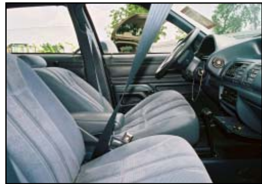
Figure 9. View of driver's seat and displaced arm rest
