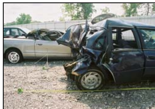
Figure 8. Lateral view showing the severe crush and trunk lid contact with the backlight header
