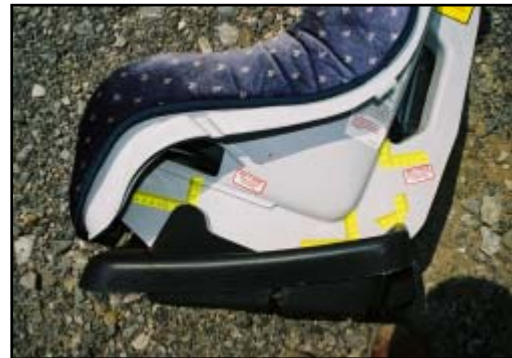
Figure 17. Left side view showing fracture and stress marks
