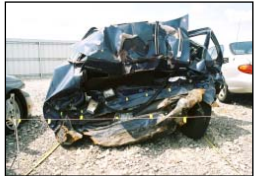
Figure 6. View of the rear damage to the Tempo
