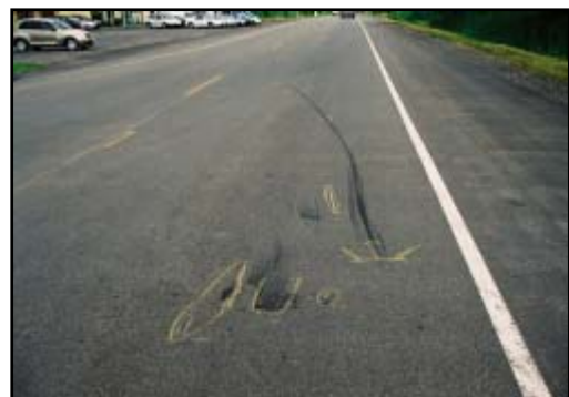
Figure 5. Close-up of point of impact and right rear tire mark
