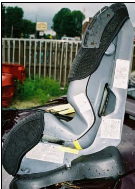
Figure 11. Loading damage to the belt path.
