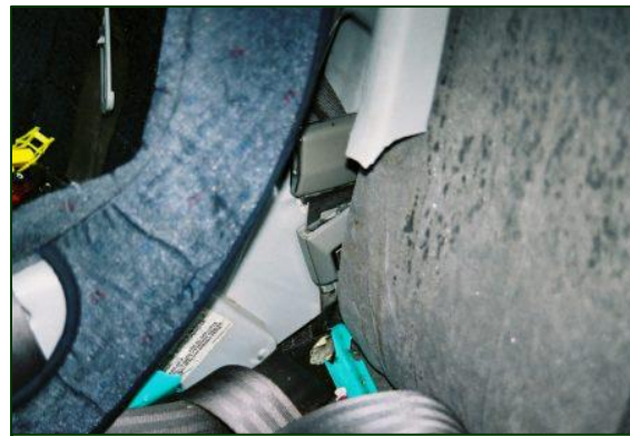
Figure 10. Released right rear safety belt buckle.
