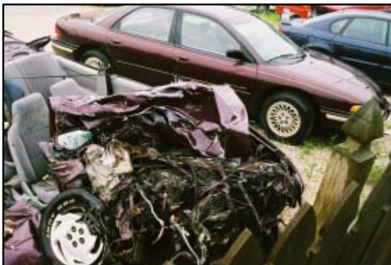
Figure 5. Overhead view of the frontal damage.
