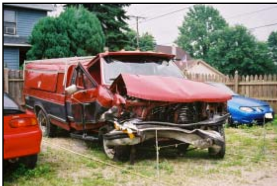
Figure 8. Resultant damage to the front of the 1993 Ford F-250.
