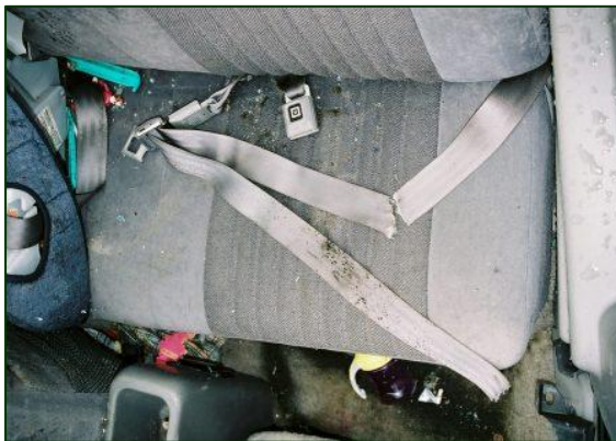
Figure 9. Cut left rear safety belt.
