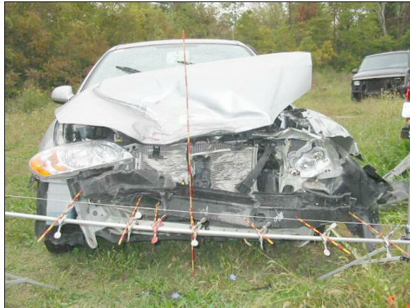
Figure 5: Case vehicle's frontal damage with contour gauge set at bumper level (case photo #17)
