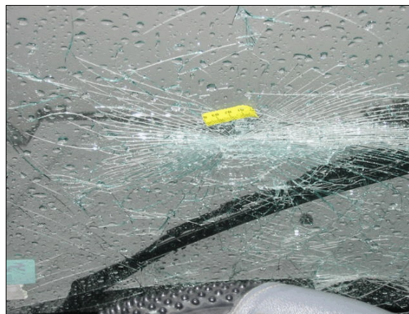
Figure 17: Close-up of left side of case vehicle's windshield glazing, directly in front of steering wheel rim, showing occupant contact evidence (case photo #53)
