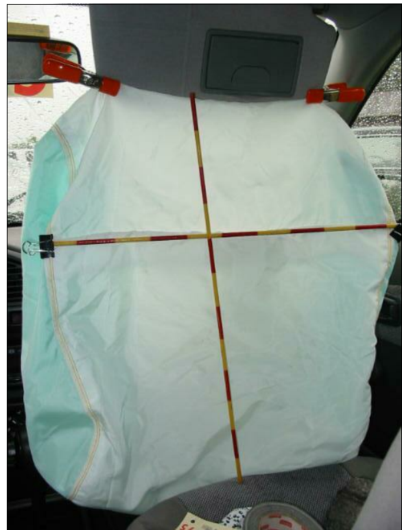
Figure 19: Case vehicle's deployed front right passenger air bag showing no apparent evidence of occupant contact on front surface (case photo #48)
