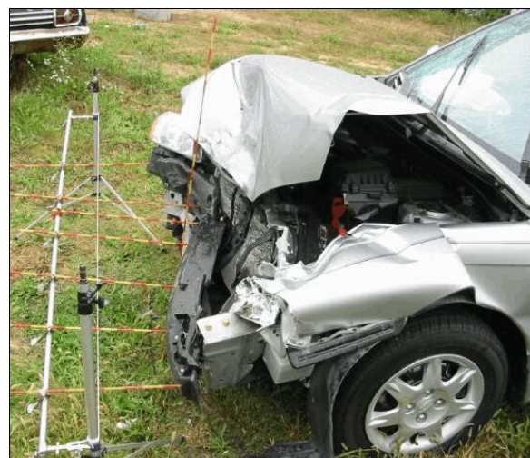
Figure 10: Reference line view from left showing case vehicle’s frontal damage with contour gauge set at bumper level (case photo #20)
