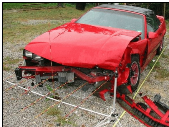
Figure 21: Elevated view of Chevrolet's frontal damage viewed from left of front with contour gauge present at bumper level; Note: bumper fascia in lower right of photo (case photo #61)
