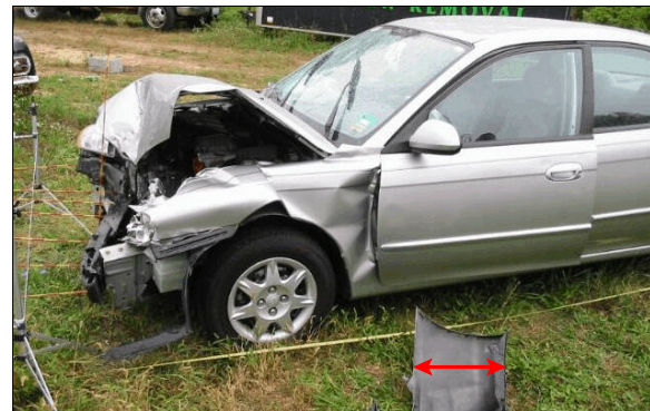
Figure 12: Case vehicle's frontal damage viewed from left front showing induced damage to hood, left fender, and driver's door; arrow indicates bumper's fascia (case photo #21)
