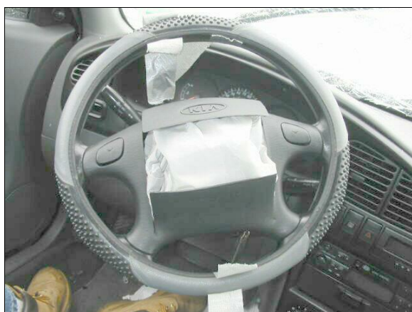
Figure 13: Elevated view of case vehicle’s steering wheel; Note: right side of steering wheel rotated forward toward left instrument panel and no obvious deformity of steering wheel’s rim and/or hub/spokes (case photo #34)
