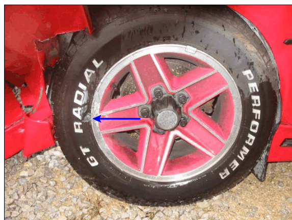
Figure 23: Chevrolet's damaged (arrow) and restricted left front wheel (case photo #63a)
