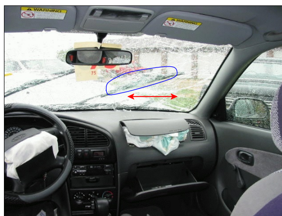
Figure 16: Case vehicle’s front right seating area showing deployed front right air bag and cracks to right side of windshield’s glazing; Note: lower crack (red arrows) is most likely from contact by front right air bag module’s cover flap while upper crack (blue line) most likely resulted from contact by driver (case photo #37)
