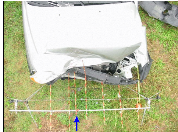
Figure 11: Overhead view of case vehicle's frontal damage with contour gauge set at bumper level (case photo #30)
