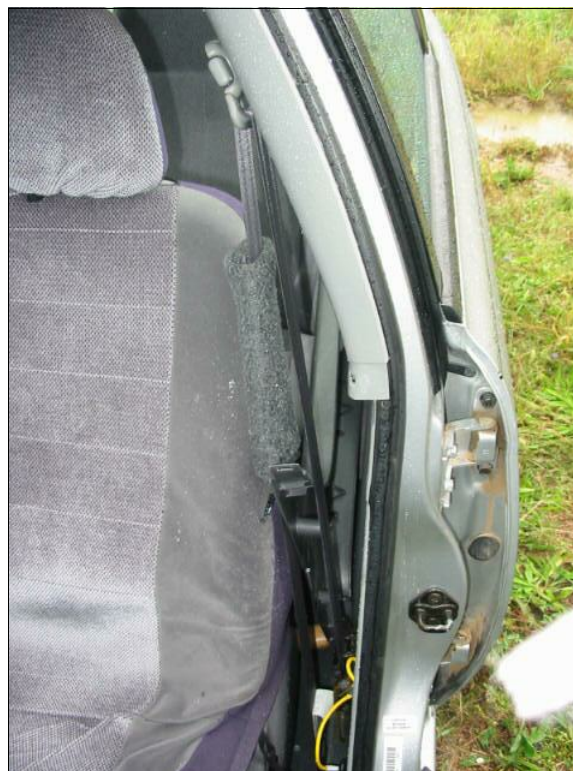
Figure 20: Rigid webbing along left "B"-pillar from case vehicle's driver safety belt indicating that pretensioner actuated while belt was not in use (case photo #54)
