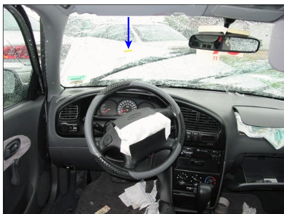
Figure 15: Case vehicle’s driver seating area showing deployed driver air bag, collapsed steering wheel, and contact (i.e., yellow tape–arrow) to left side of windshield’s glazing (case photo #35)
