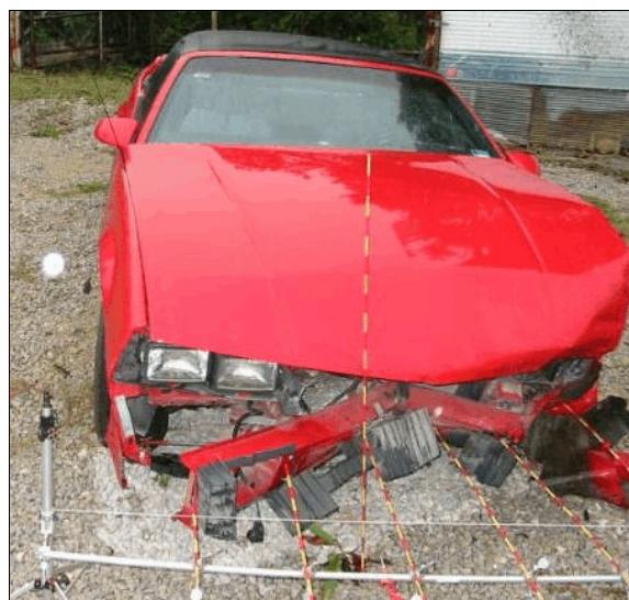
Figure 22: Elevated view from front right of Chevrolet's frontal damage with contour gauge present at bumper level (case photo #71)
