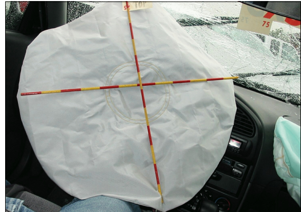
Figure 18: Case vehicle's deployed driver air bag showing no apparent occupant contact evidence on front surface of air bag's fabric (case photo #40)
