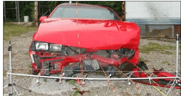
Figure 6: Chevrolet's frontal damage with contour gauge set at bumper level (case photo #58)
