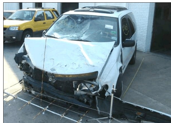
Figure 3: Elevated view of Nissan's overlapping frontal damage viewed from left of front; Note: front left half damage most likely from initial impact with barrels (case photo #54)
