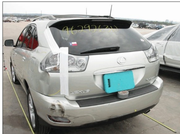
Figure 9: Damage to back portion of case vehicle's left rear quarter panel and bumper from impact with barrels during clockwise rotation to final rest (case photo #17)
