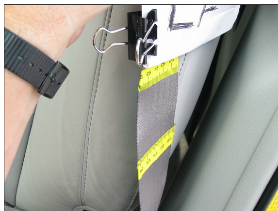
Figure 19: Loading evidence (i.e., scuffs/friction burns) on webbing of torso portion case vehicle's driver safety belt (case photo #44)
