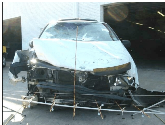
Figure 22: Overlapping damage to Nissan’s front from impact with barrels and case vehicle; Note: contour gauge positioned along actual bumper (case photo #52)
