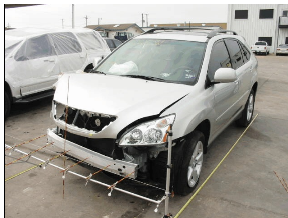
Figure 7: Case vehicle’s frontal damage from impact with Nissan viewed from left of front; Note: lesser damage to front left resulted from contact with Nissan’s right front door as case vehicle wrapped around Nissan’s right side (case photo #13)
