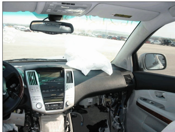
Figure 12: Case vehicle's front right passenger seating area showing no apparent occupant contact evidence (case photo #28)
