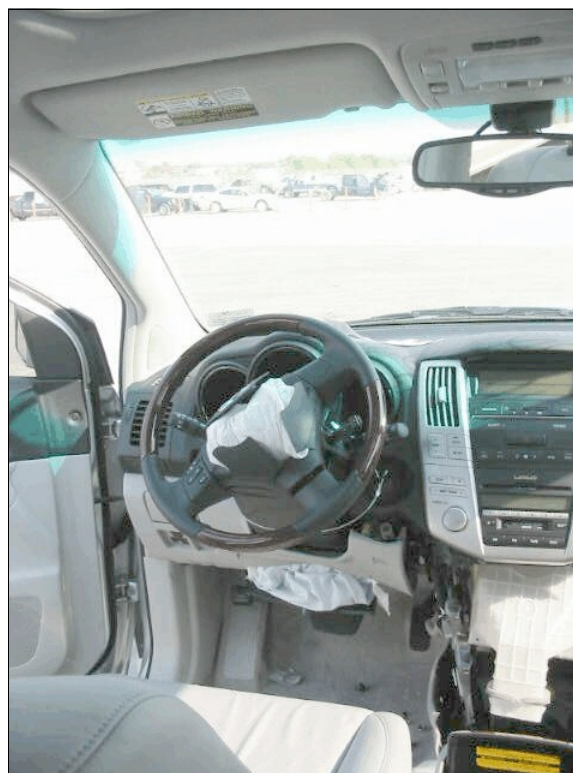
Figure 11: Vertical view of case vehicle's driver seating area showing no apparent evidence of occupant contact (case photo #26a)
