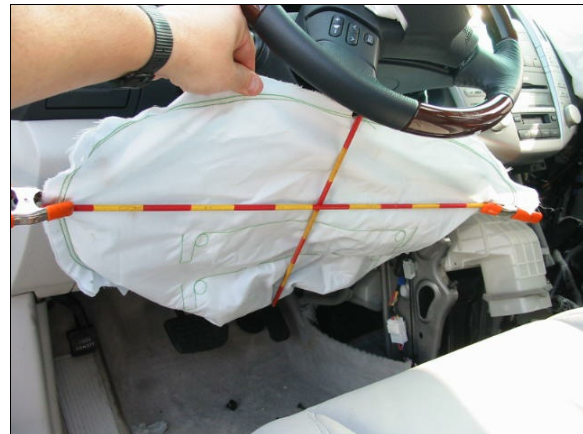
Figure 18: Seat level view of case vehicle's deployed, under column-mounted, knee bolster air bag showing no residual occupant contact evidence (case photo #42)
