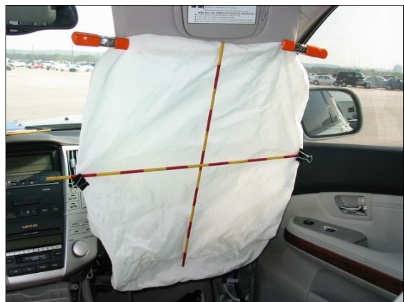
Figure 16: Case vehicle's deployed front right passenger air bag showing no apparent evidence of occupant contact (case photo #35)
