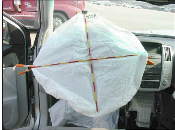
Figure 14: Case vehicle's deployed driver air bag showing no obvious occupant contact evidence (case photo #32)
