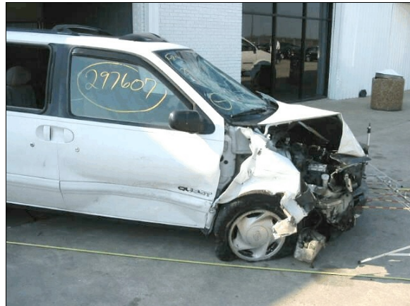
Figure 8: Nissan's frontal and right side damage viewed from right front; Note: displacement of right front wheel assembly and damage on right front door caused by wrap-around damage from impact with case vehicle (case photo #60)
