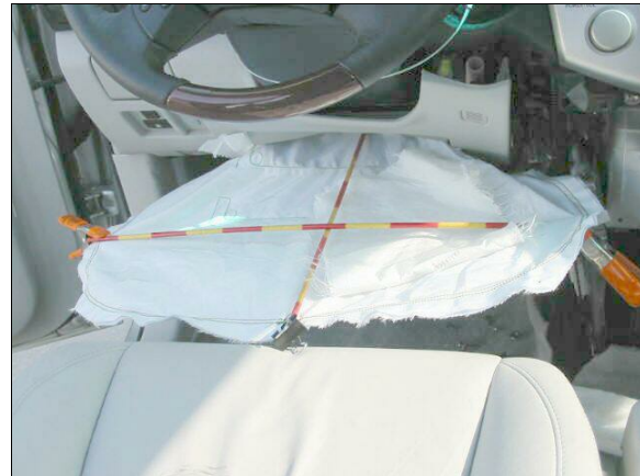
Figure 17: Elevated view of case vehicle's deployed, under column-mounted, knee bolster air bag showing no residual evidence of occupant contact (case photo #41)
