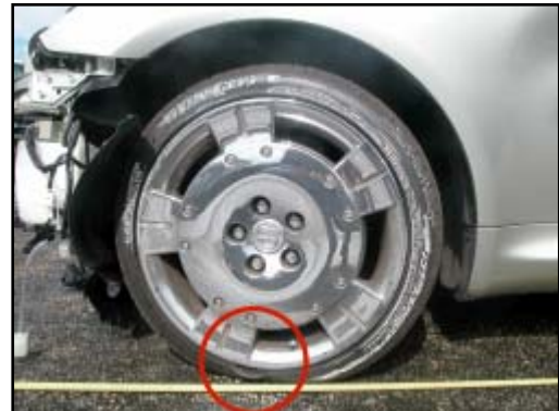
Figure 4. Left front wheel/tire showing minor sidewall damage
