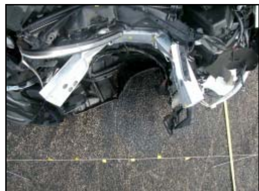
Figure 6. Overhead view of crushed bumper beam
