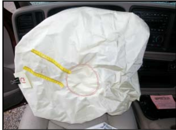
Figure 12: Driver air bag. Note the 90 degree CCW rotation of the steering wheel.
