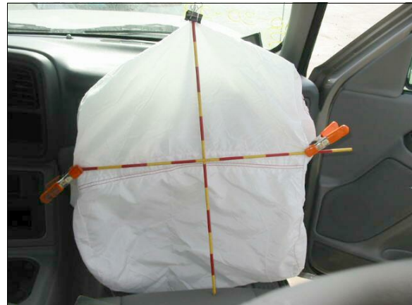
Figure 16: Case vehicle's deployed front right passenger air bag showing no apparent evidence of occupant contact on front surface (case photo #38)
