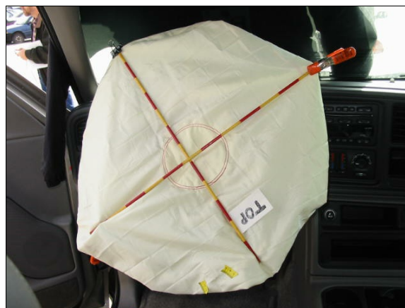
Figure 14: Case vehicle's deployed driver air bag showing only slight scuff near 1 o'clock position; Note: air bag rotated approximately 140 degrees clockwise (case photo #33)
