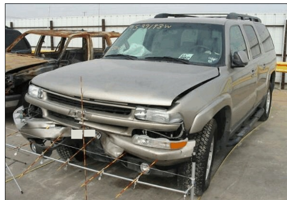
Figure 5: Case vehicle's frontal damage from impact with Ford viewed from left of front with contour gauge set at bumper level (case photo #13)
