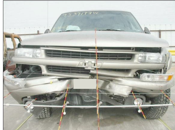
Figure 4: Case vehicle's frontal damage from impact with Ford; Note: contour gauge positioned at bumper level (case photo #11)
