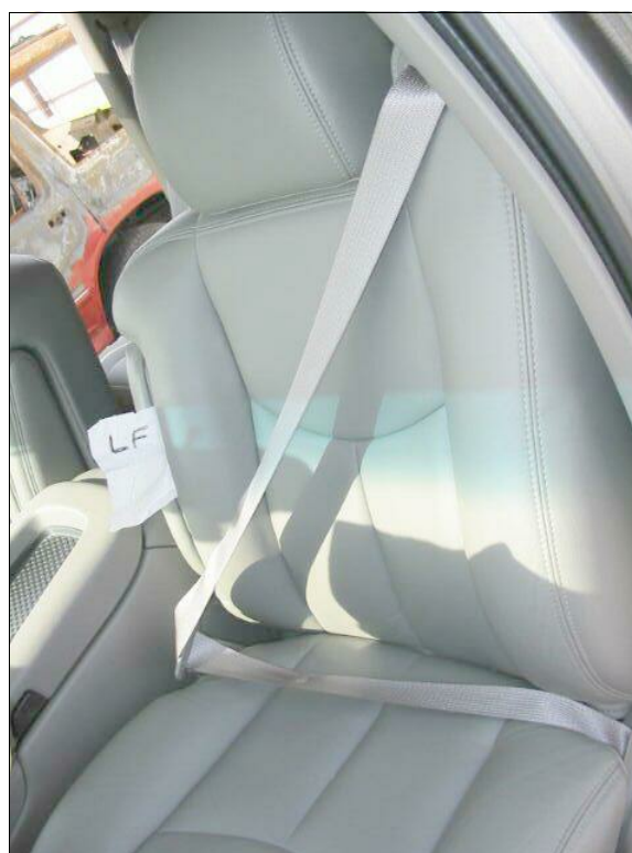
Figure 17 Case vehicle's driver seat and integrated safety belts showing no apparent loading evidence on webbing (case photo #42)
