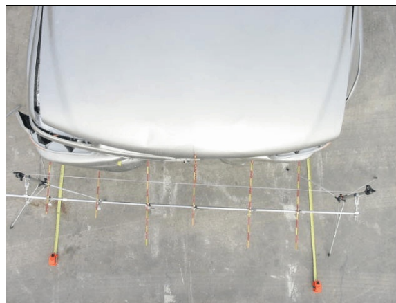
Figure 9: Overhead view of frontal damage to case vehicle from impact with Ford (case photo #23)
