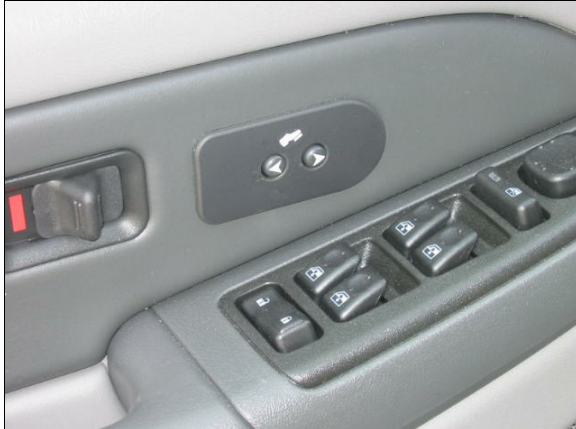
Figure 7: Buttons on interior surface of case vehicle's driver door controlling adjustable foot pedals (case photo #45)
