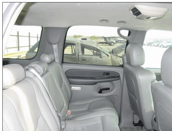
Figure 13: Case vehicle's second seating area viewed from right showing no apparent evidence of occupant contact and second seat center's integrated three-point lap and shoulder safety belt system (case photo #51)
