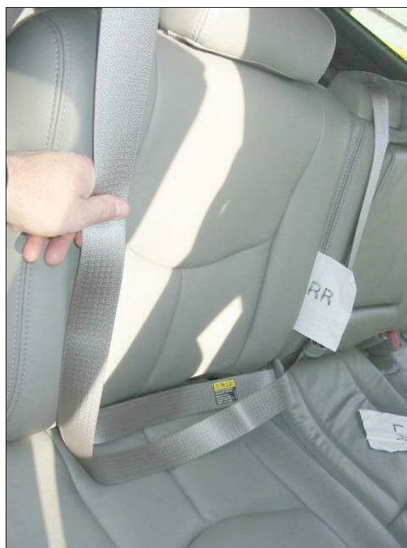
Figure 20: Case vehicle's second right seat cushion, adjustable head restraint, and safety belts showing no apparent loading evidence on webbing (case photo #55)
