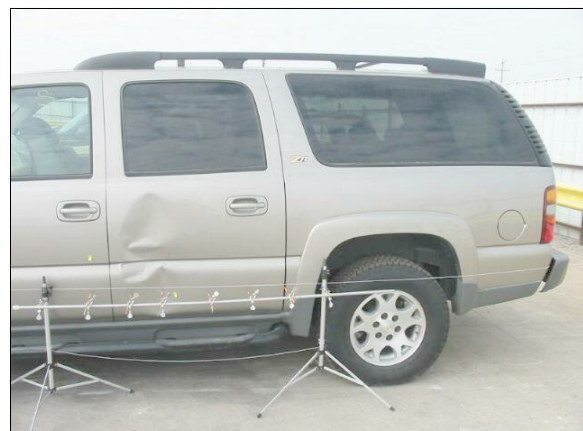
Figure 6: Case vehicle's side slap damage, primarily to left rear door (case photo #16)
