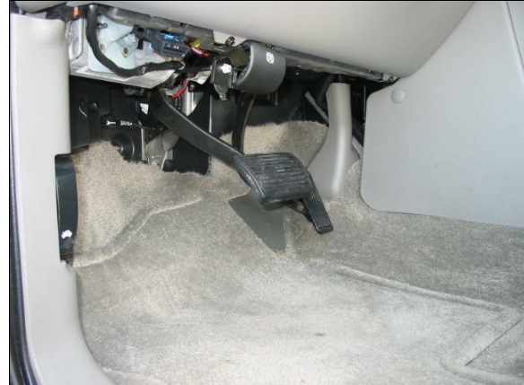
Figure 8: Adjustable foot controls for case vehicle's driver—exact position of pedals is unknown (case photo #46)
