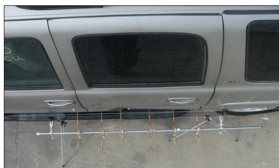
Figure 10: Overhead view of side slap damage, primarily to case vehicle’s left rear door (case photo #15a)
