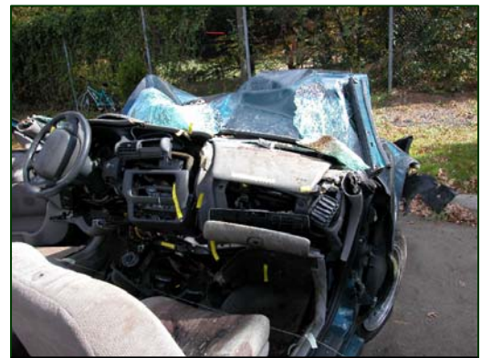
Figure 9. Overall view of front right area and the passenger's contact points.
