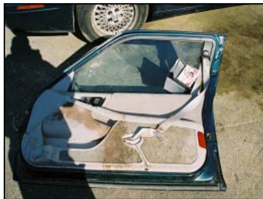
Figure 13. Front right 3-point automatic safety belt system.
