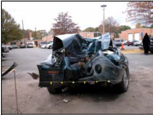
Figure 6. Frontal damage from the large diameter tree.
