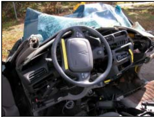
Figure 11. Non-deployed driver's frontal air bag.
