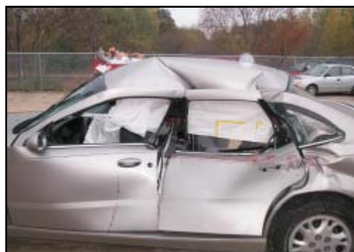
Figure 18. Outboard view of left IC showing areas of scuff marks
