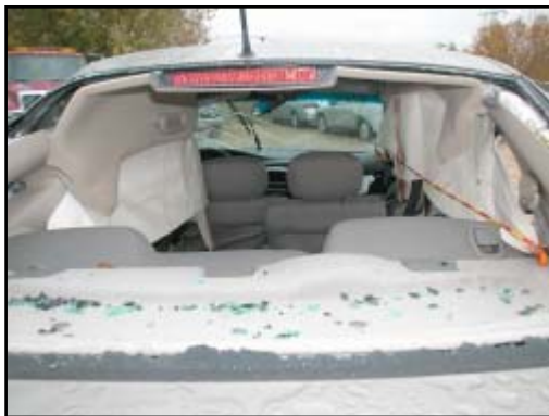
Figure 16. View from backlight showing left and right side IC's
