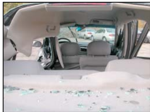
Figure 8. View through the backlight of the Saturn L200 showing lateral intrusions
