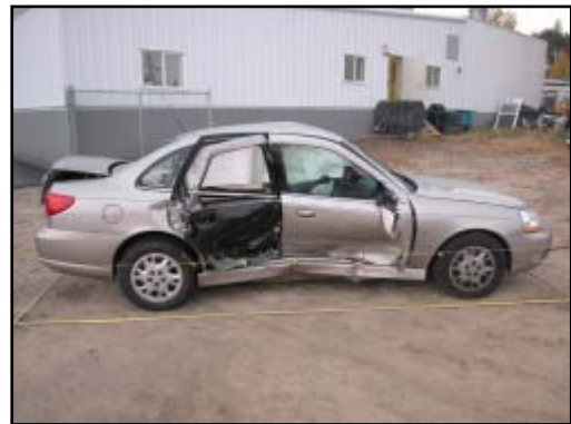
Figure 6. Right side damage to the Saturn L200
