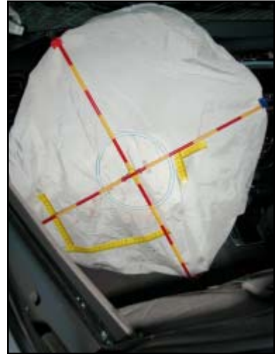
Figure 13. Deployed driver's air bag (steering wheel rotated 60 degrees CW)
