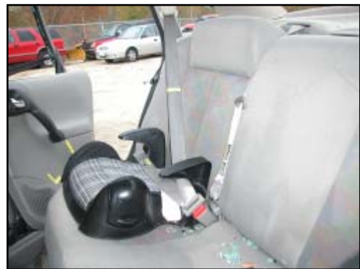
Figure 12. BPB in position with the vehicle's safety belt
