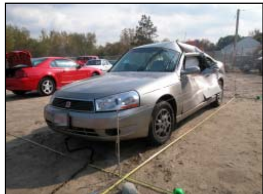
Figure 7. View of the left side damage to the Saturn L200
