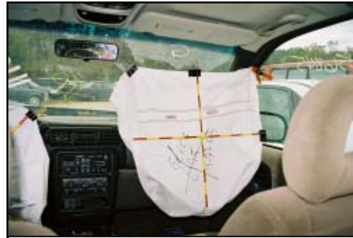
Figure 16. Deployed front right frontal air bag.
