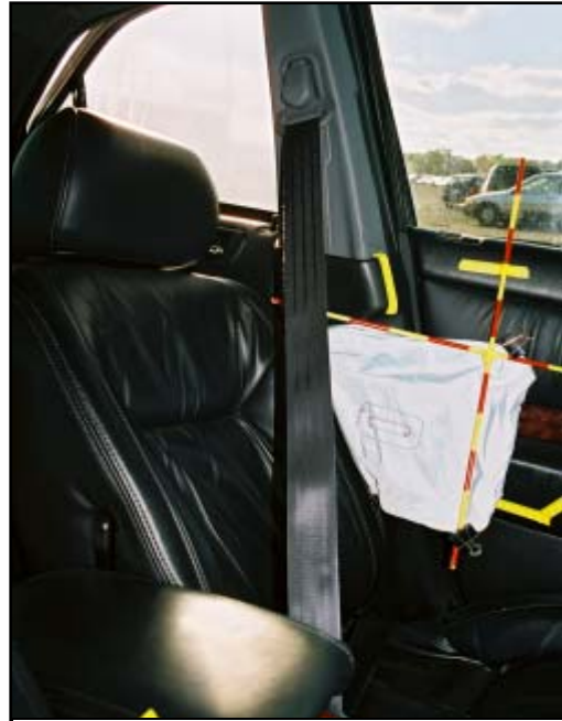
Figure 10. Deployed driver's side impact air bag.
