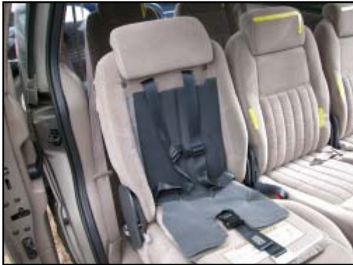
Figure 18. Integrated child safety seat in the second row right of the 1998 Pontiac Transport.
