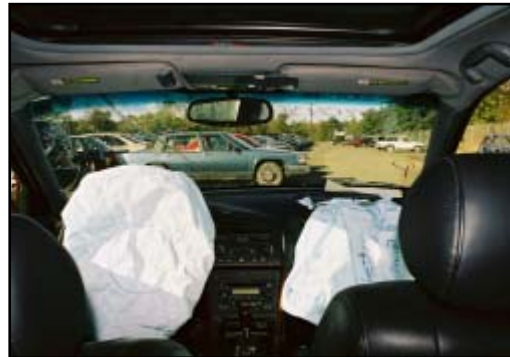
Figure 11. Deployed frontal air bags.
