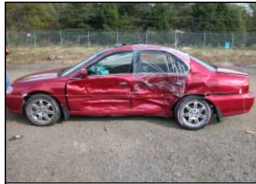
Figure 6. Damage profile of 2000 Acura 3.2 TL.
