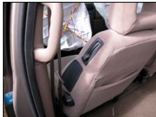
Figure 17. Non-deployed driver's side impact air bag.
