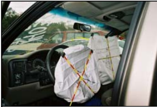
Figure 15. Deployed driver's frontal air bag.
