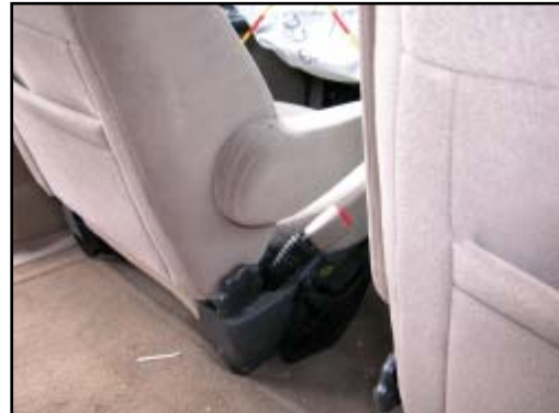
Figure 14. Fired driver's buckle pretensioner.
