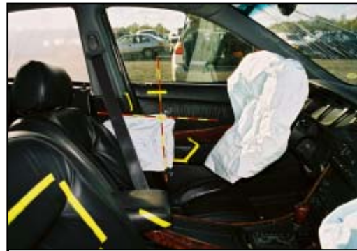
Figure 7. Interior damage to 2000 Acura 3.2 TL.
