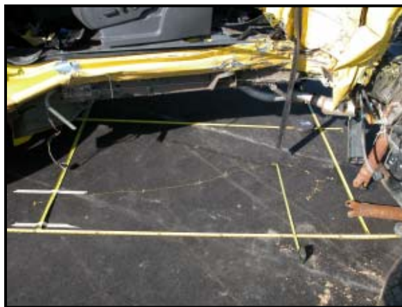
Figure 6: View of the crush profile of the left sill.
