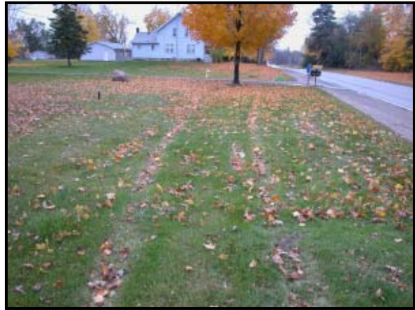
Figure 3: Trajectory view of the yaw marks leading to the point of impact.
