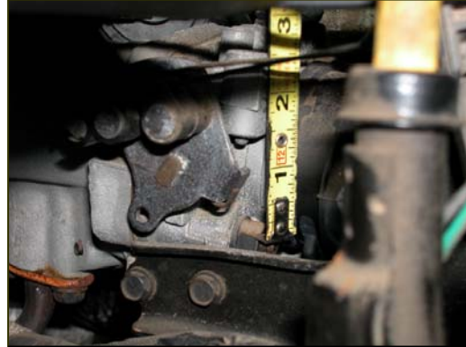
Figure 13. Open throttle position resulting from the frayed cable.
