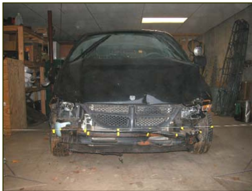
Figure 10. Frontal damage to the Dodge Caravan.
