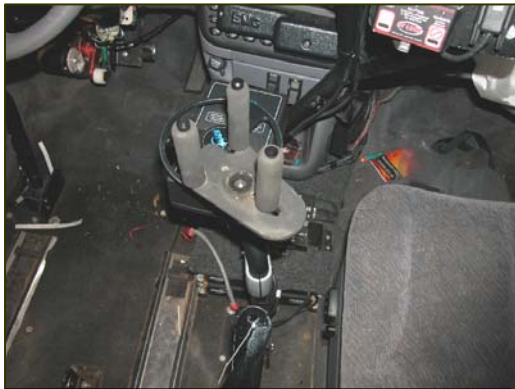
Figure 5. Remote steering assembly with tri-pin device.
