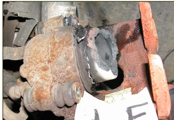
Figure 17. Deteriorated left front brake caliper piston and boot seal.
