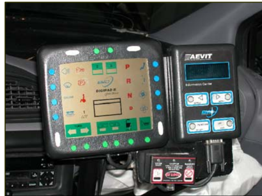
Figure 6. DigiPad II control display with the AEVIT information system.
