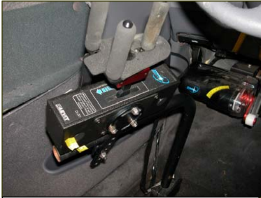
Figure 3. Adaptive hand control for the throttle and brake functions.
