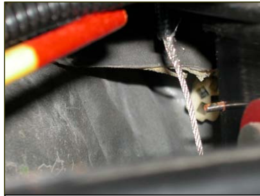
Figure 15. Frayed adaptive control throttle cable.
