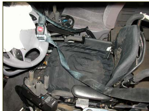
Figure 3. Retrofitted safety belt system in the adjusted position worn by the driver.
