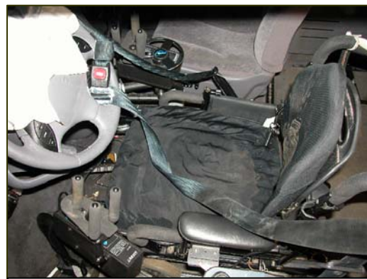
Figure 12. Driver’s seated position and the adjusted position of the retrofitted safety belt.
