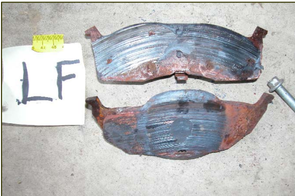
Figure 16. Left front disc brake pads. Note deflection of lower (piston side) backer plate.
