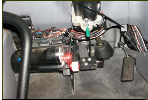
Figure 4. Servo motor and cable routed to the OEM accelerator pedal.
