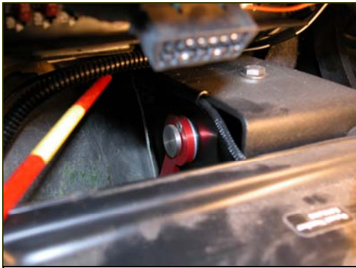
Figure 14. Cable and servo motor cam arm centered in image.
