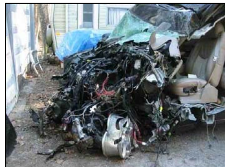
Figure 6 - Frontal damage to the 2004 GMC Yukon XL.
