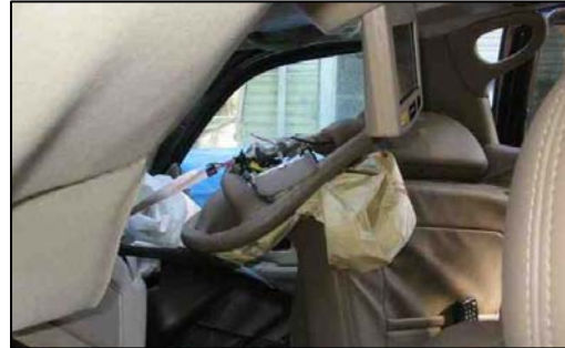
Figure 13 - Steering assembly and compressed front right seat.
