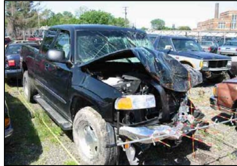
Figure 4 – Frontal damage to 2003 GMC Sierra.
