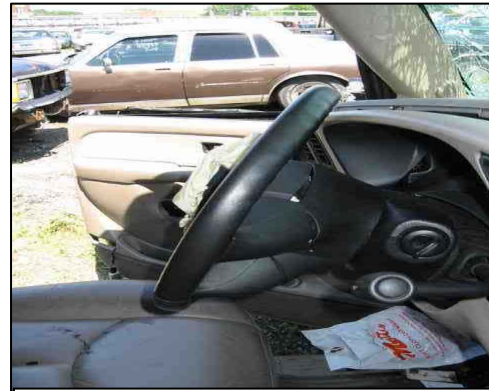
Figure 7 – Lateral view of steering wheel rim deformation.
