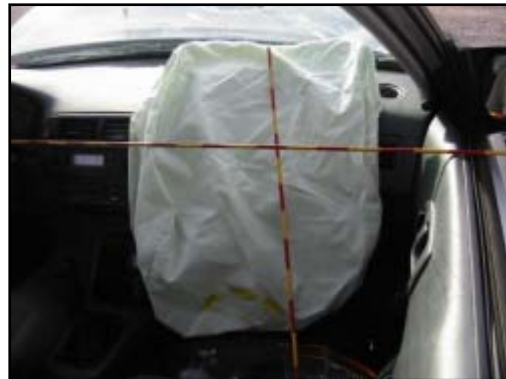
Figure 8. Deployed front right air bag.
