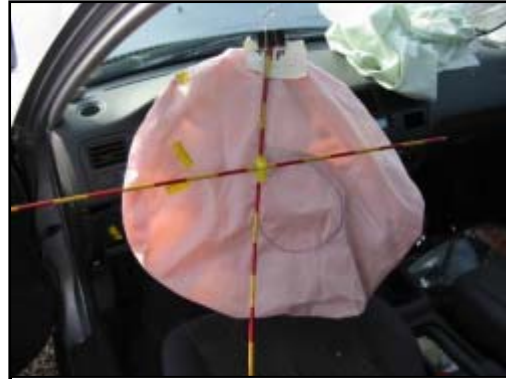
Figure 7. Deployed driver's frontal air bag. The area of occupant contacts was to the upper left quadrant.
