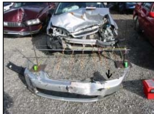
Figure 5. Resultant frontal damage from the impact with the Pontiac.
