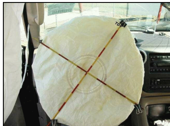
Figure 6: Front of driver's air bag; left safety canopy is partially visible on the left in this photos
