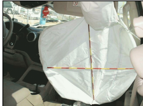
Figure 7: Front of front right passenger's air bag; right side canopy is hanging from above in this view
