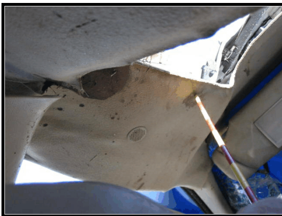
Figure 11. Possible head contact to roof
