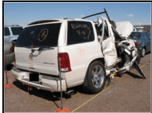
Figure 7. Overview of roof and right side intrusion
