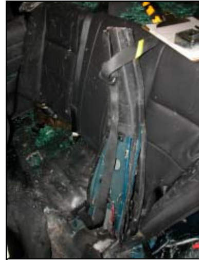
Figure 7. View of separated left B-pillar and driver's safety belt webbing
