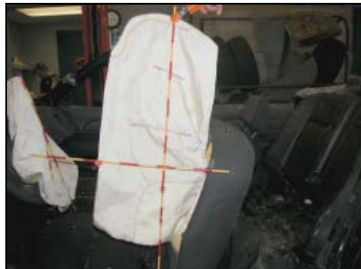
Figure 10. View of deployed driver's side impact air bag
