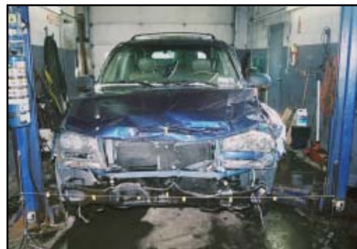
Figure 6. Frontal damage to the 2002 Chevrolet Trailblazer
