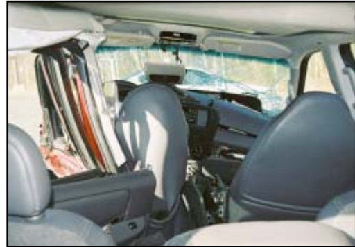
Figure 7. View of interior from the rear showing intrusions
