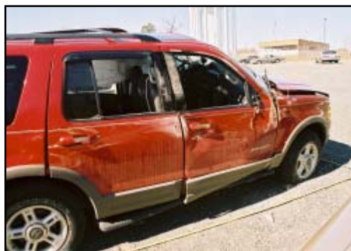
Figure 6. View of the right side trip-over damage to the Ford Explorer
