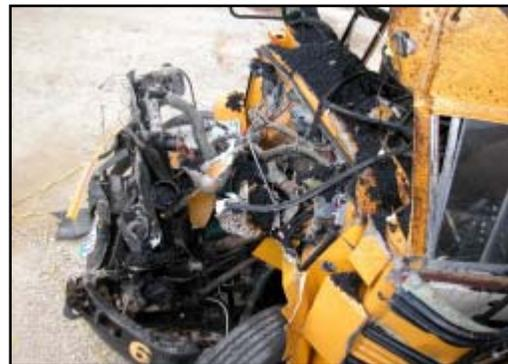
**Figure 8. Overhead view of cowl deformation.**
