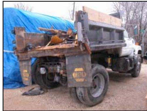
**Figure 13. Damage area of the struck dump truck.**
