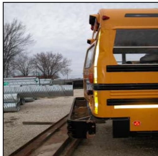
**Figure 10. View of body chassis separation at the rear.**
