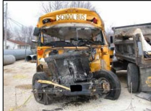
**Figure 7. Frontal damage to subject school bus and bumper level crush profile.**
