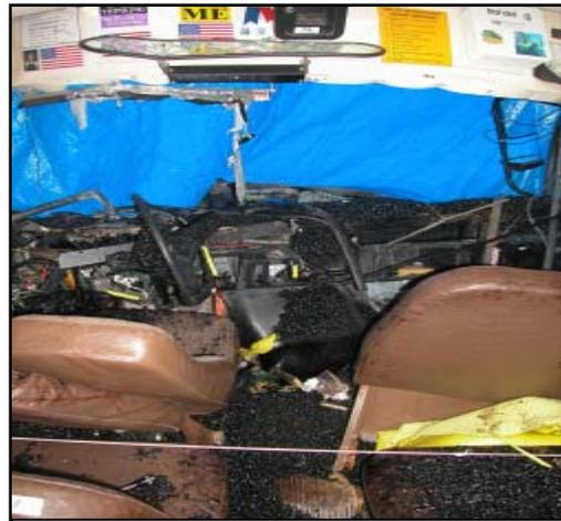
**Figure 12. Center instrument panel contacts from the 15-year-old female passenger and final rest area for this occupant.**
