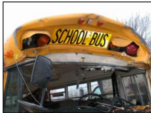
**Figure 9. Windshield header crush profile.**
