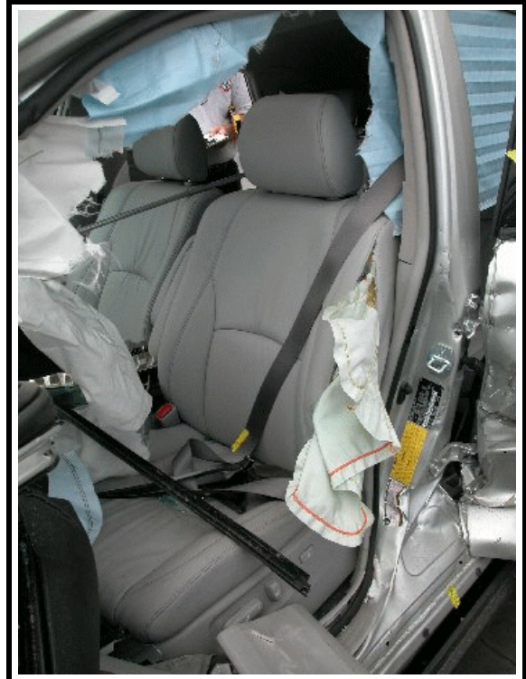
Figure 4. View showing spooled out webbing
