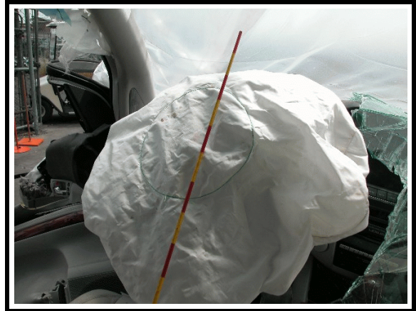
Figure 7. View showing deployed drivers air bag
