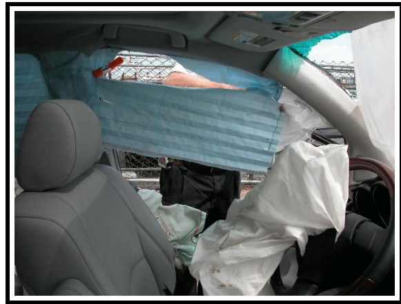
Figure 9. View showing deployed left side curtain shield air bag
