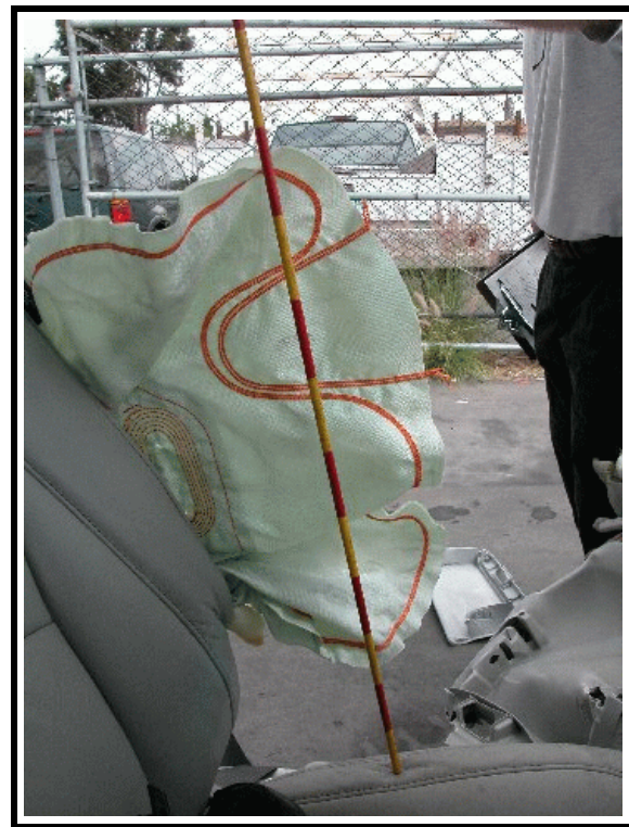
Figure 10. View showing deployed left side thoracic air bag
