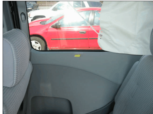
Figure 7: Intrusion and contact mark (yellow tape) on interior surface of right rear sliding door adjacent to second seating row.
