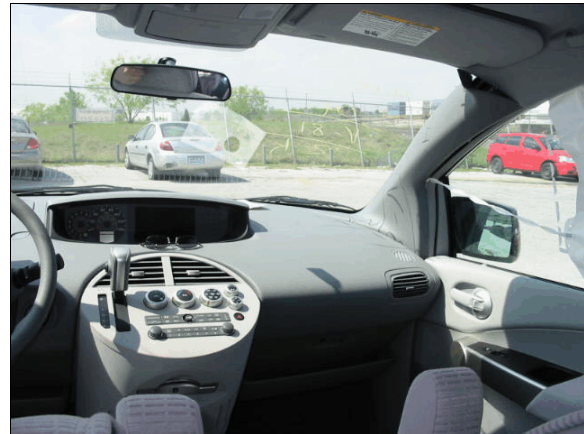
Figure 10: Case vehicle's front right seating area, front right passenger air bag located in top of right instrument panel
