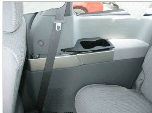
Figure 8: Damage and intrusion of case vehicle's side-panel into back right seat area.
