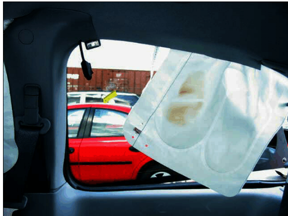
Figure 6: Yellow tape shows occupant contact mark on case vehicle's back right window, note make-up transfer on side curtain air bag
