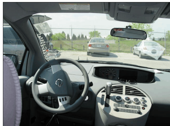
Figure 9: Case vehicle's driver seating area showing non-deployed driver air bag and no occupant contact evidence to interior surfaces
