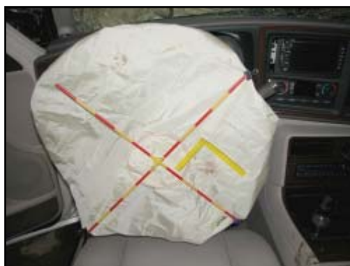
Figure 8. Deployed driver's air bag
