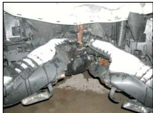
Figure 5. Close-up of maximum crush and fractured bumper beam
